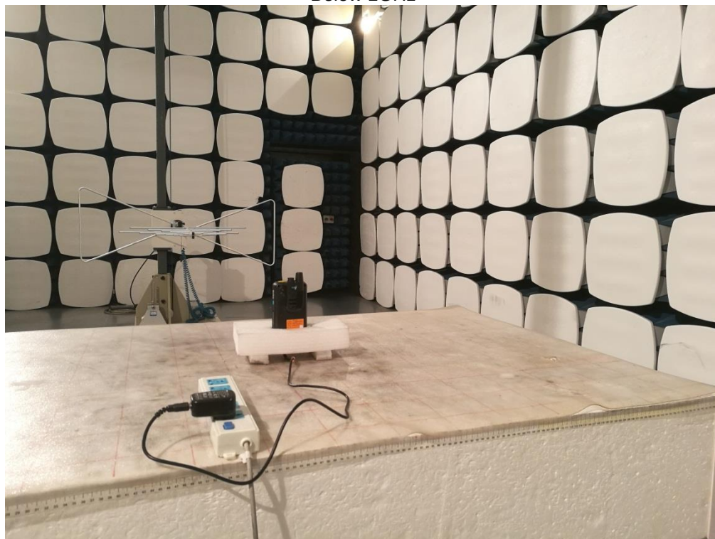
Radiated Spurious Emission Below 1GHz
