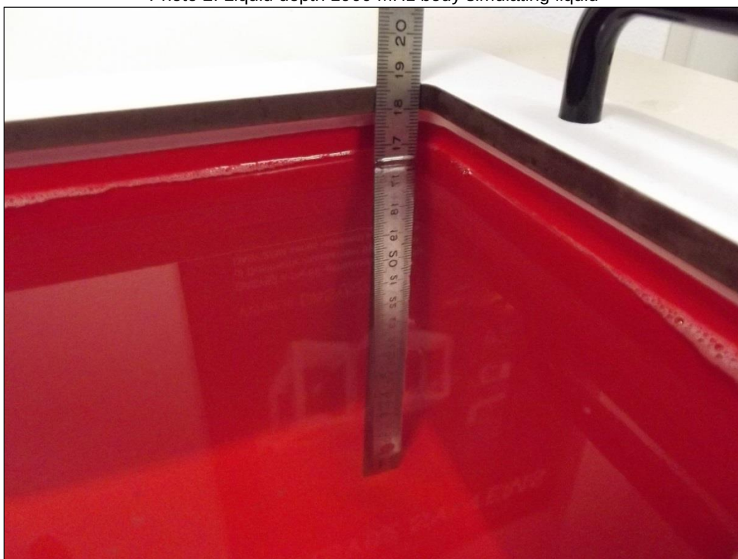
Photo 2: Liquid depth 1900 MHz body simulating liquid
