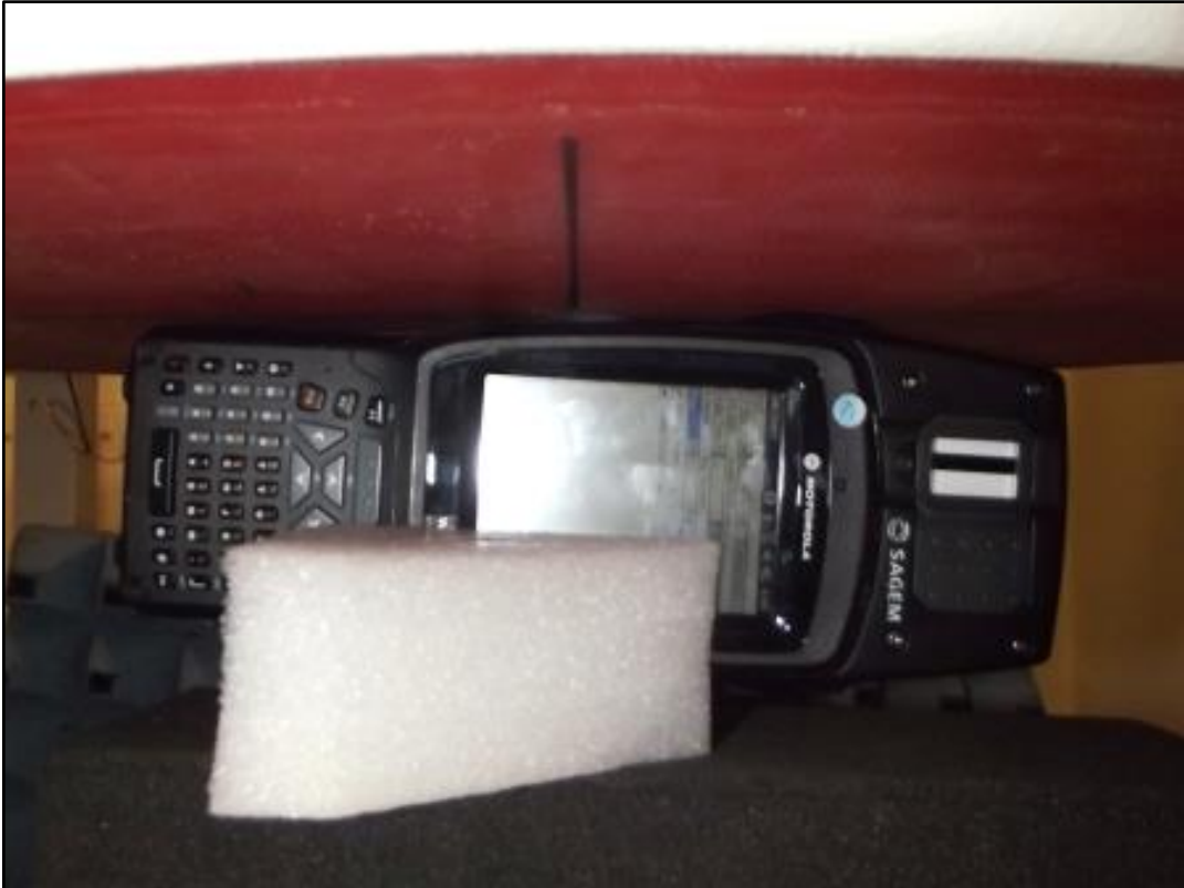
Photo 13: Test position left side with 0 mm distance
