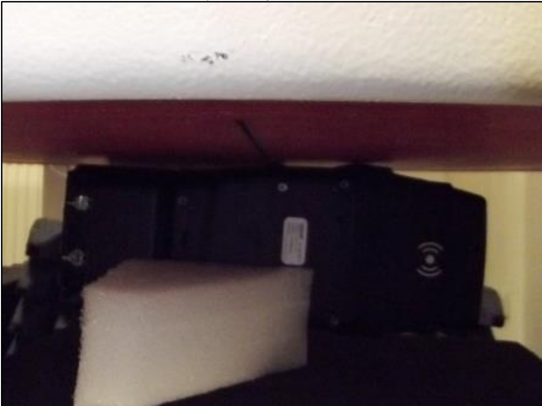
Photo 14: Test position right side with 0 mm distance
