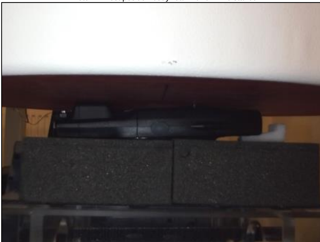
Photo 12: Test position body rear with 0 mm distance
