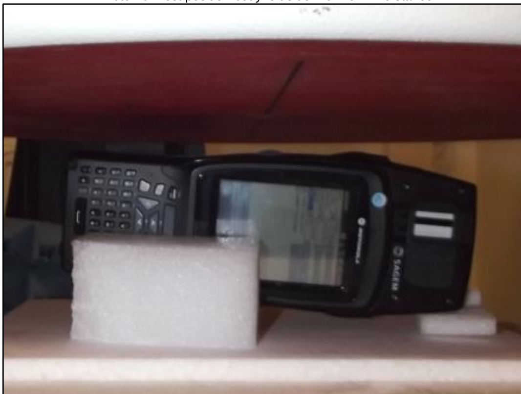
Photo 10: Test position body left side with 20 mm distance
