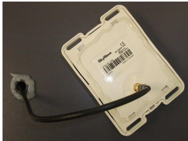
Figure 29 Apply Silicone to Hole in Asset
