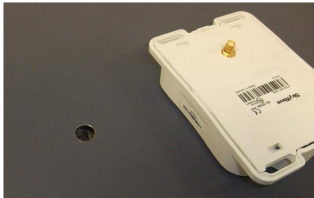
Figure 27 Drill Mounting Hole
