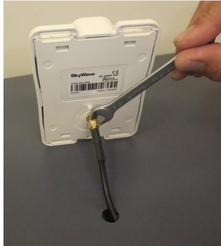
Figure 28 Attach Cable to Antenna
