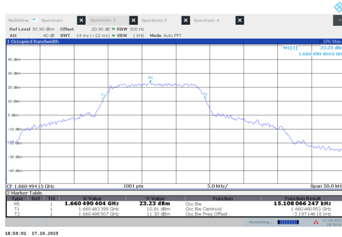
Figure 7.1-27: 99 % bandwidth on high channel for waveform Z
