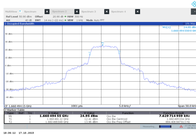
Figure 7.1-21: 99 % bandwidth on high channel for waveform Y
