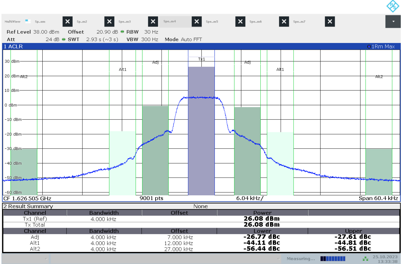
Figure 7.3-2: Conducted band edge spurious emissions outside assigned bandwidth – Waveform Y, low channel
