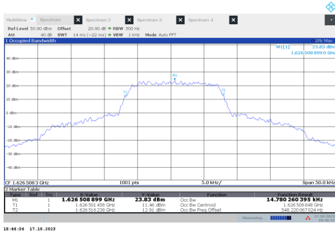
Figure 7.1-25: 99 % bandwidth on low channel for waveform Z
