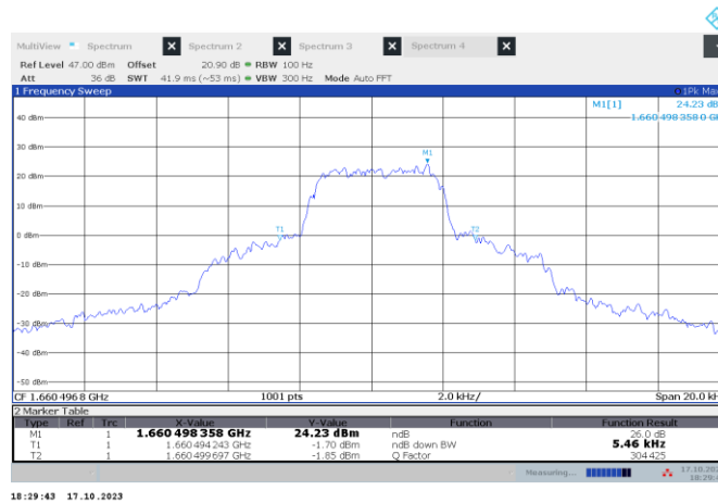
Figure 7.1-18: 26 dB bandwidth on high channel for waveform T
