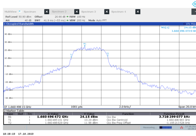
Figure 7.1-15: 99 % bandwidth on high channel for waveform T
