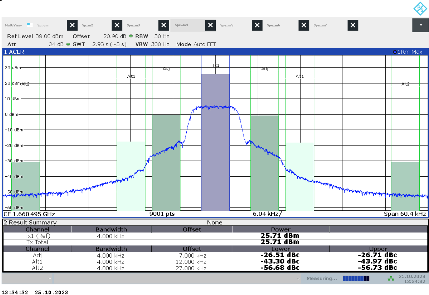
Figure 7.3-2: Conducted band edge spurious emissions outside assigned bandwidth – Waveform Y, high channel
