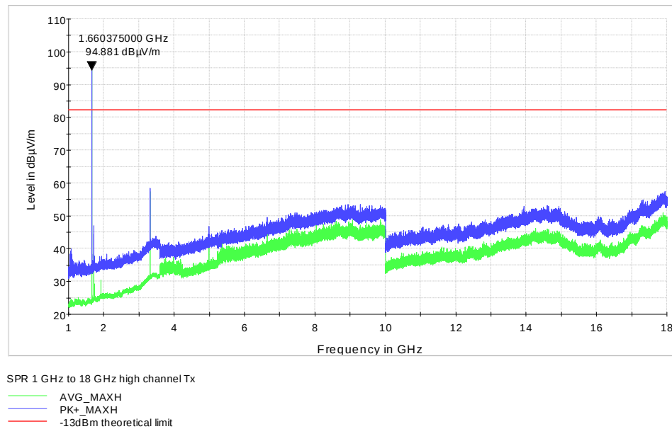
Figure 7.3-18: Radiated spurious emissions 1 – 18 GHz for sub-band 1, high channel waveform T
