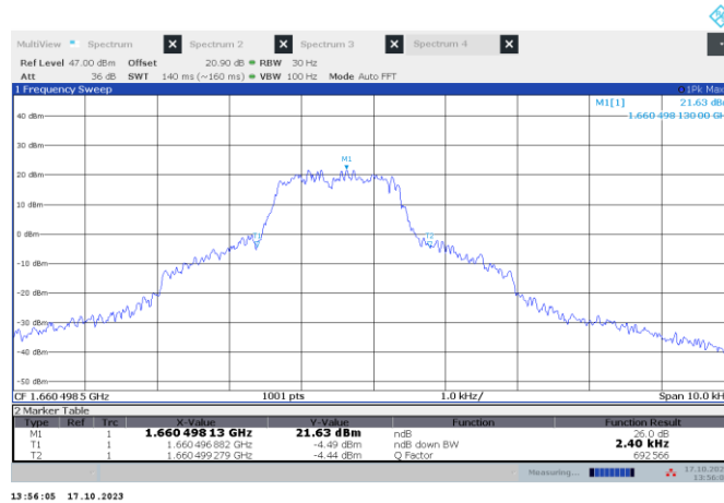
Figure 7.1-12: 26 dB bandwidth on high channel for waveform K
