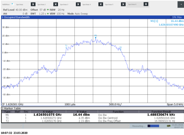
Figure 8.1-1: 99 % bandwidth on low channel
