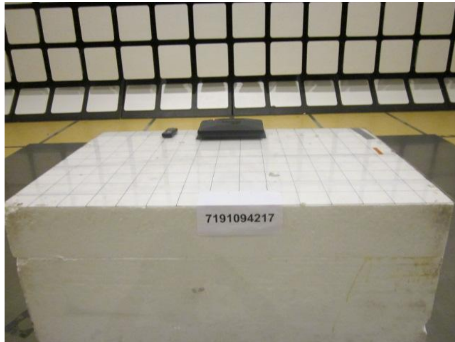
Radiated Emissions Test Setup (Front View)
