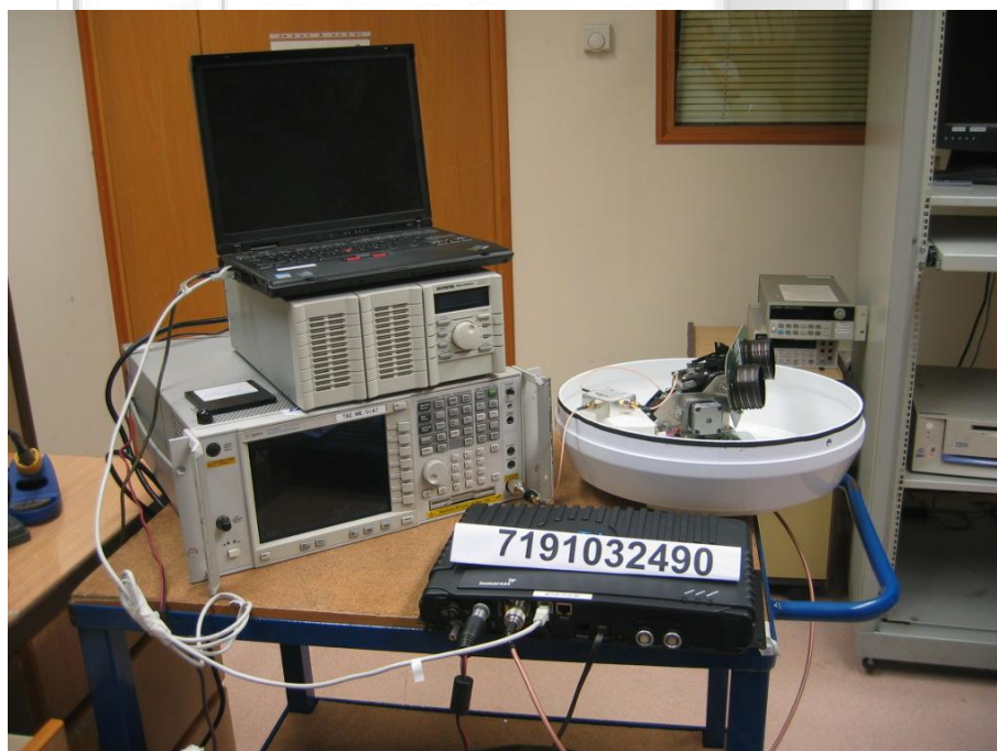
Unwanted Emissions at Antenna Terminal Test Setup
