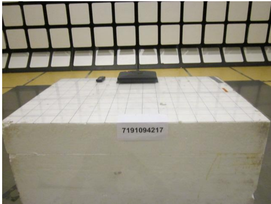
Radiated Emissions Test Setup (Front View)
