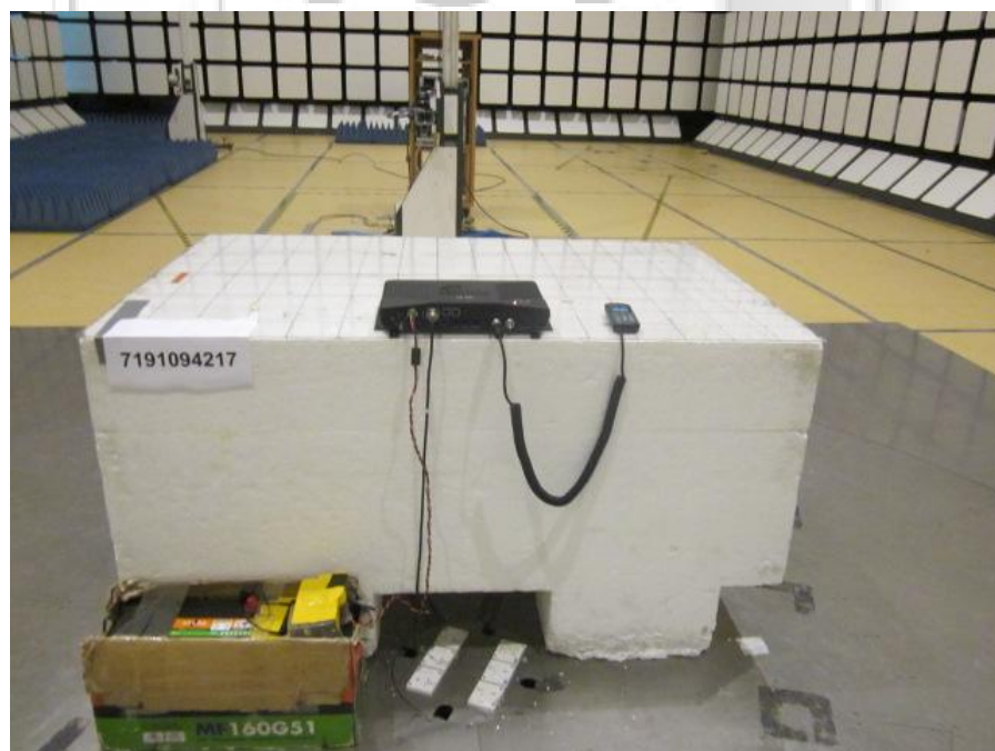
Radiated Emissions Test Setup (Rear View)
