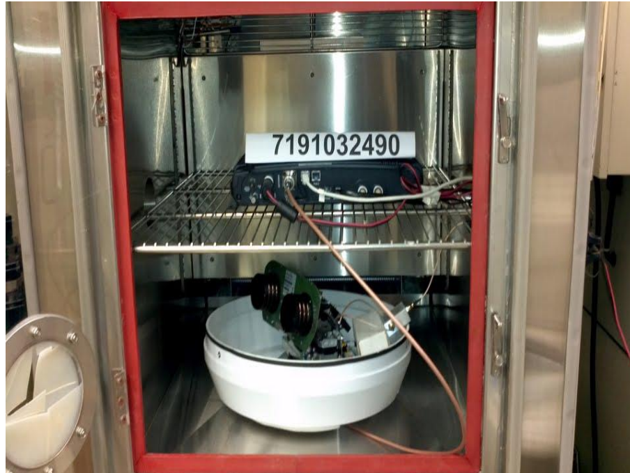
Frequency Stability (Temperature Variation) Test Setup
