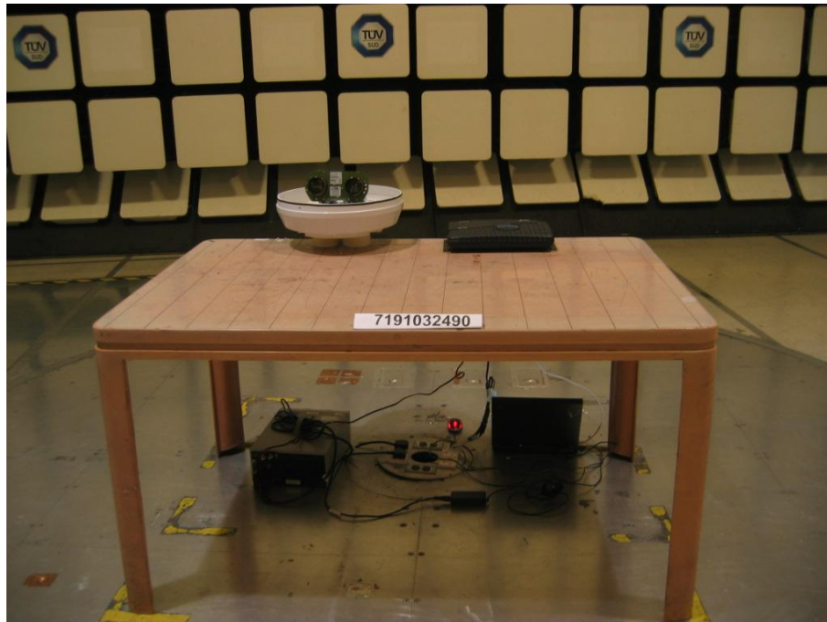
Radiated Spurious Emissions Test Setup (Front View)
