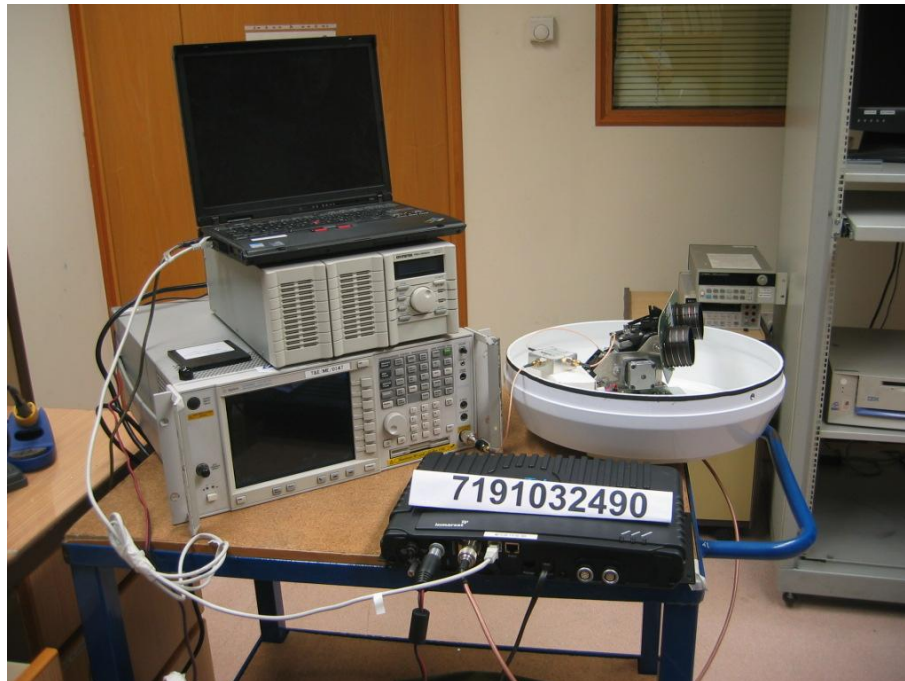
RF Output Power Test Setup
