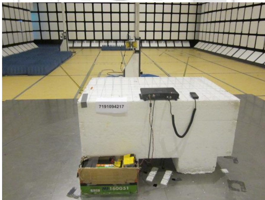
Radiated Emissions Test Setup (Rear View)
