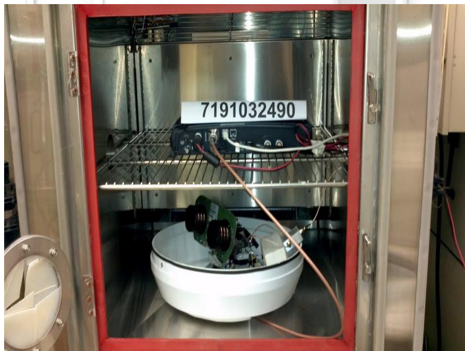
Frequency Stability (Voltage Variation) Test Setup
