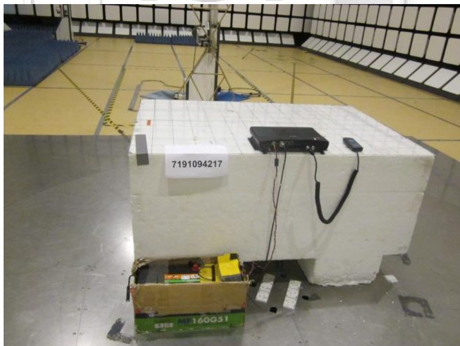
Radiated Emissions Test Setup (Rear View)
