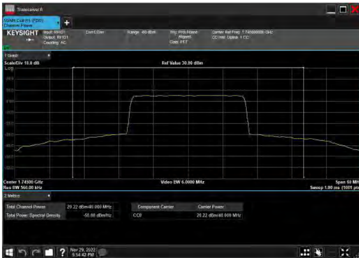
DC_2A_n66A_10MHz|40MHz_15kHz_1880MHz|1745MHz_Q PSK|CP-OFDM QPSK_RB12@0|RB108@54
