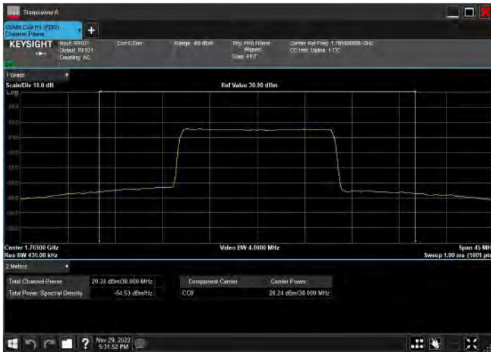
DC_2A_n66A_10MHz|30MHz_15kHz_1905MHz|1765MHz_Q PSK|CP-OFDM 256 QAM_RB12@38|RB80@40
