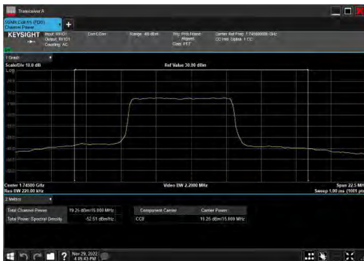
DC_2A_n66A_10MHz|15MHz_15kHz_1880MHz|1745MHz_Q PSK|DFT-s-OFDM 256 QAM_RB12@0|RB36@18
