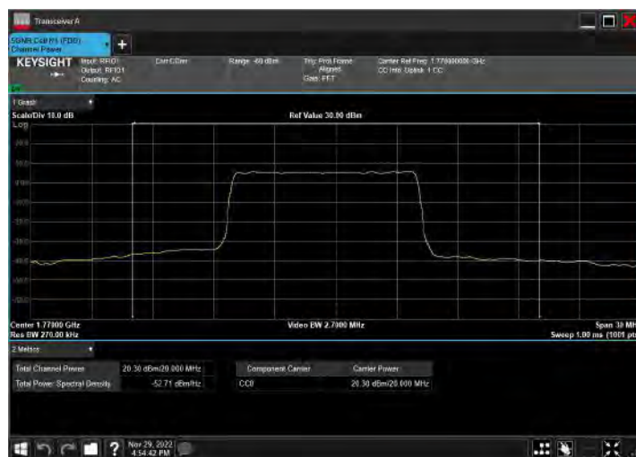
DC_2A_n66A_10MHz|20MHz_15kHz_1905MHz|1770MHz_Q PSK|DFT-s-OFDM 64 QAM_RB12@38|RB50@25
