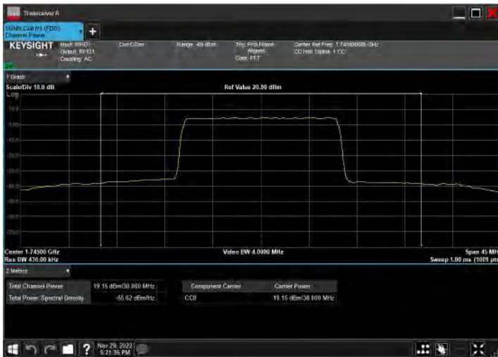
DC_2A_n66A_10MHz|30MHz_15kHz_1880MHz|1745MHz_Q PSK|CP-OFDM 256 QAM_RB12@0|RB80@40
