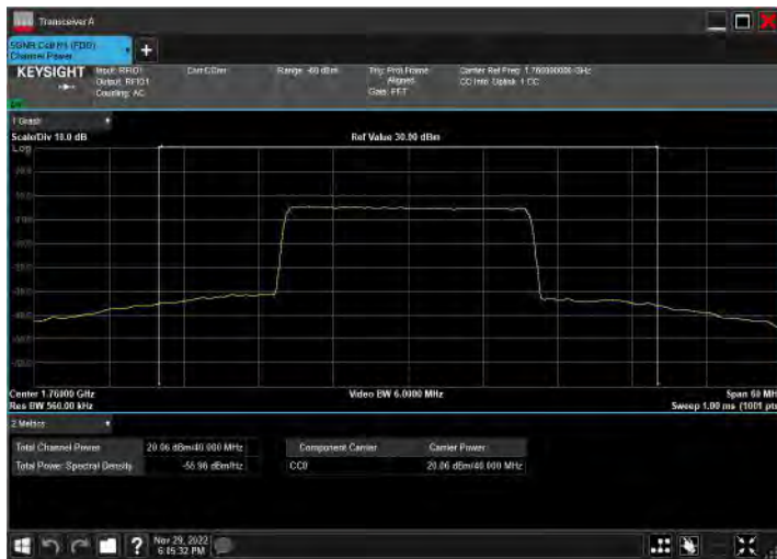
DC_2A_n66A_10MHz|40MHz_15kHz_1905MHz|1760MHz_Q PSK|DFT-s-OFDM 16 QAM_RB12@38|RB108@54
