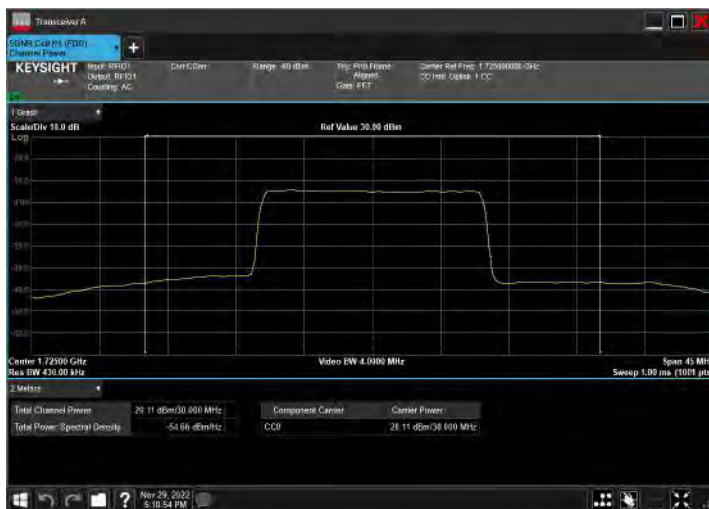
DC_2A_n66A_10MHz|30MHz_15kHz_1855MHz|1725MHz_Q PSK|CP-OFDM 64 QAM_RB12@0|RB80@40
