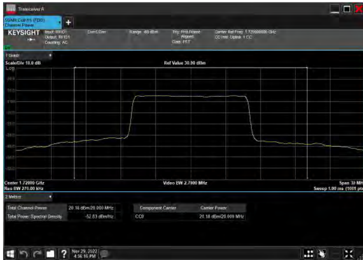
DC_2A_n66A_10MHz|20MHz_15kHz_1855MHz|1720MHz_Q PSK|CP-OFDM 256 QAM_RB12@0|RB53@26
