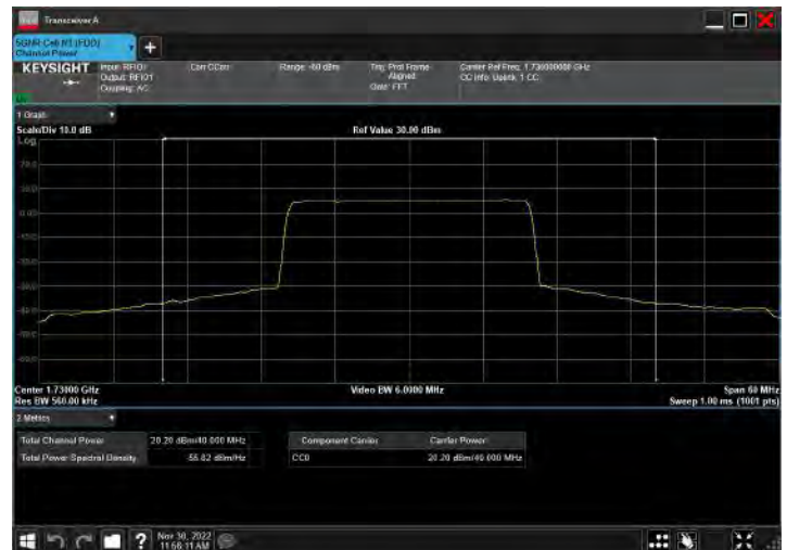
DC_5A_n66A_10MHz|40MHz_15kHz_829MHz|1730MHz_QP SK|CP-OFDM QPSK_RB12@0|RB108@54
