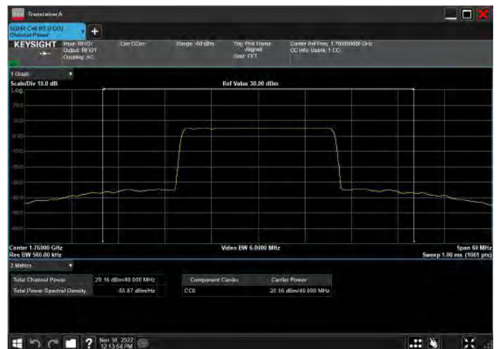
DC_5A_n66A_10MHz|40MHz_15kHz_844MHz|1760MHz_QP SK|DFT-s-OFDM 64 QAM_RB12@38|RB108@54
