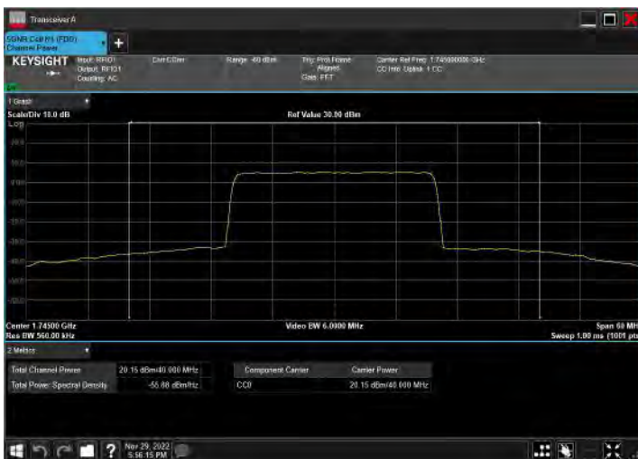
DC_2A_n66A_10MHz|40MHz_15kHz_1880MHz|1745MHz_Q PSK|CP-OFDM 64 QAM_RB12@0|RB108@54
