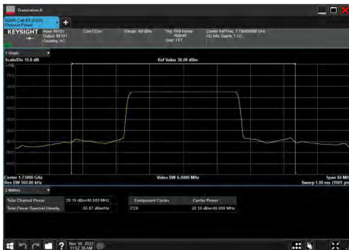
DC_5A_n66A_10MHz|40MHz_15kHz_829MHz|1730MHz_QP SK|DFT-s-OFDM PI/2 BPSK_RB12@0|RB108@54
