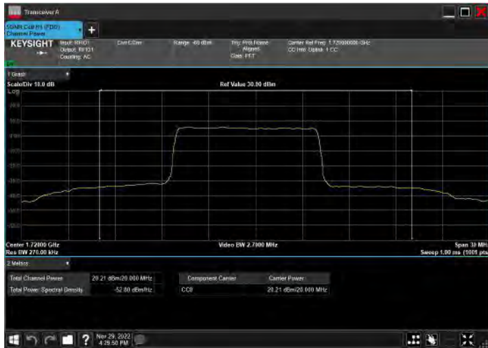
DC_2A_n66A_10MHz|20MHz_15kHz_1855MHz|1720MHz_Q PSK|DFT-s-OFDM 64 QAM_RB12@0|RB50@25
