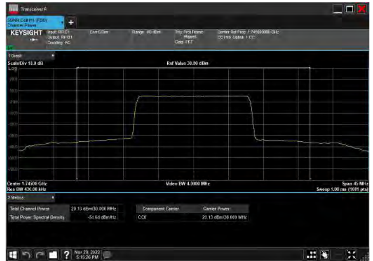
DC_2A_n66A_10MHz|30MHz_15kHz_1880MHz|1745MHz_Q PSK|DFT-s-OFDM 64 QAM_RB12@0|RB80@40
