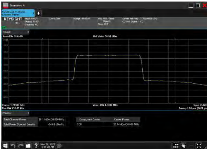
DC_2A_n66A_10MHz|30MHz_15kHz_1880MHz|1745MHz_Q PSK|DFT-s-OFDM 16 QAM_RB12@0|RB80@40
