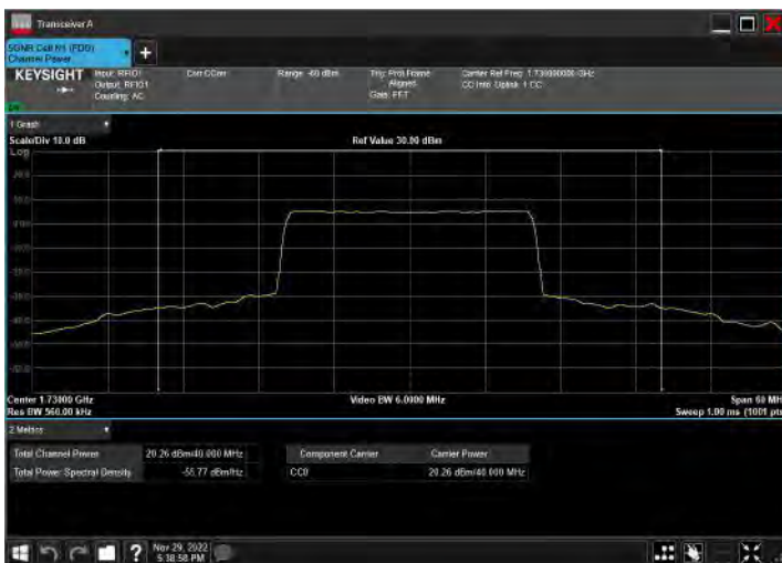
DC_2A_n66A_10MHz|40MHz_15kHz_1855MHz|1730MHz_Q PSK|DFT-s-OFDM PI/2 BPSK_RB12@0|RB108@54
