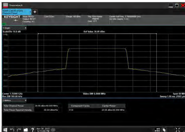
DC_5A_n66A_10MHz|40MHz_15kHz_844MHz|1760MHz_QP SK|DFT-s-OFDM 16 QAM_RB12@38|RB108@54
