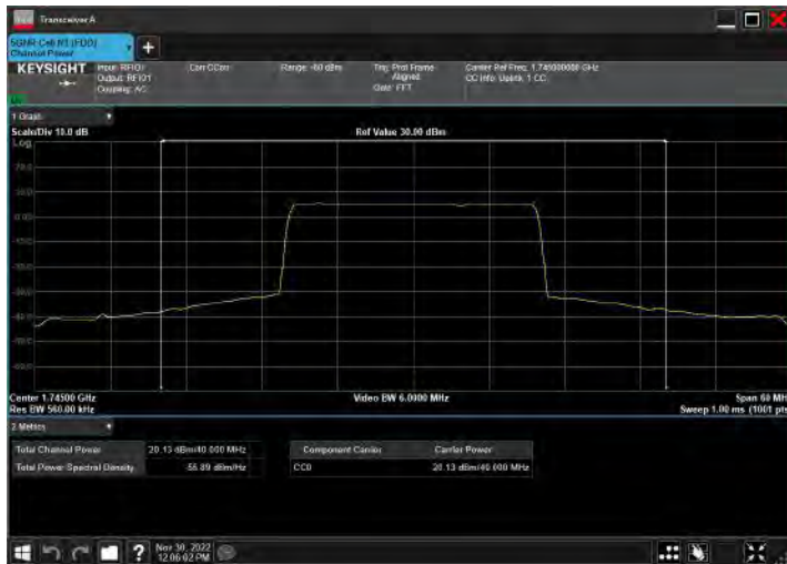
DC_5A_n66A_10MHz|40MHz_15kHz_836.5MHz|1745MHz_Q PSK|CP-OFDM QPSK_RB12@0|RB108@54
