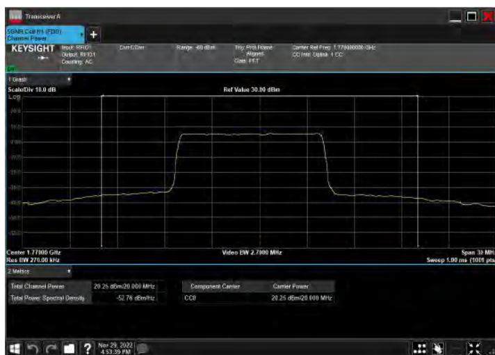
DC_2A_n66A_10MHz|20MHz_15kHz_1905MHz|1770MHz_Q PSK|DFT-s-OFDM 16 QAM_RB12@38|RB50@25
