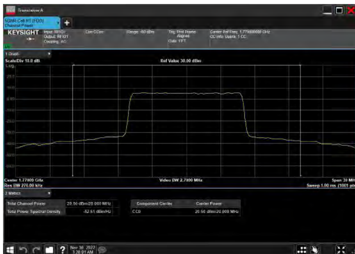
DC_5A_n66A_10MHz|20MHz_15kHz_844MHz|1770MHz_QP SK|CP-OFDM 64 QAM_RB12@38|RB53@26
