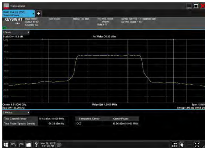
DC_2A_n66A_10MHz|10MHz_15kHz_1855MHz|1715MHz_Q PSK|CP-OFDM 256 QAM_RB12@0|RB26@13
