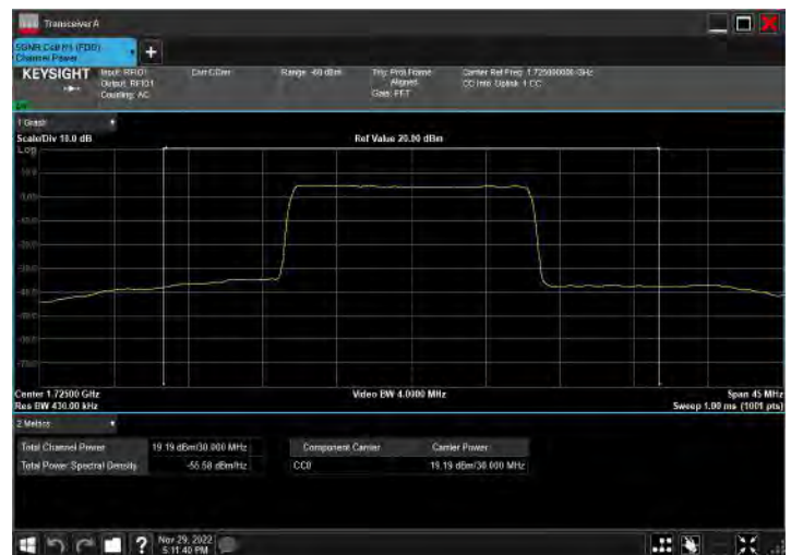
DC_2A_n66A_10MHz|30MHz_15kHz_1855MHz|1725MHz_Q PSK|CP-OFDM 256 QAM_RB12@0|RB80@40
