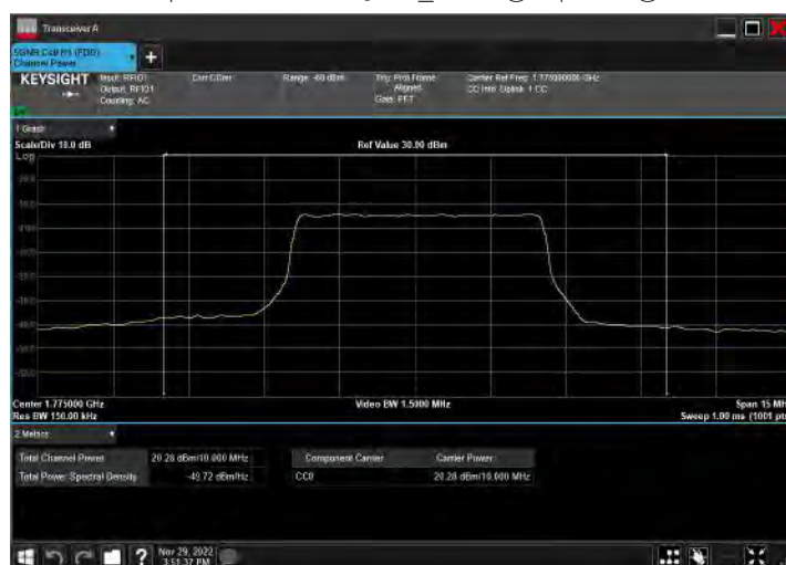
DC_2A_n66A_10MHz|10MHz_15kHz_1905MHz|1775MHz_Q PSK|CP-OFDM 16 QAM_RB12@38|RB26@13
