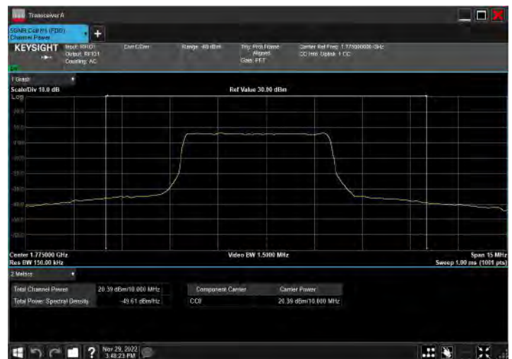
DC_2A_n66A_10MHz|10MHz_15kHz_1905MHz|1775MHz_Q PSK|DFT-s-OFDM 64 QAM_RB12@38|RB25@12
