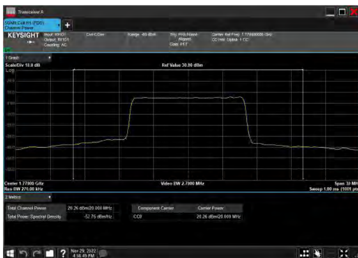
DC_2A_n66A_10MHz|20MHz_15kHz_1905MHz|1770MHz_Q PSK|CP-OFDM 64 QAM_RB12@38|RB53@26
