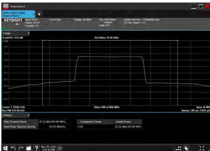
DC_2A_n66A_10MHz|30MHz_15kHz_1855MHz|1725MHz_Q PSK|DFT-s-OFDM 16 QAM_RB12@0|RB80@40
