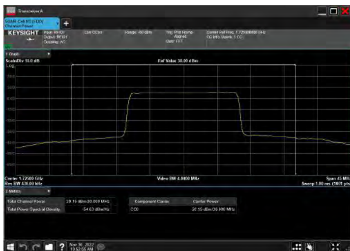
DC_5A_n66A_10MHz|30MHz_15kHz_829MHz|1725MHz_QP SK|CP-OFDM 64 QAM_RB12@0|RB80@40
