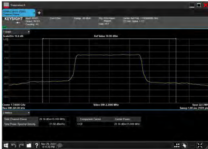
DC_2A_n66A_10MHz|15MHz_15kHz_1880MHz|1745MHz_Q PSK|CP-OFDM 256 QAM_RB12@0|RB39@19
