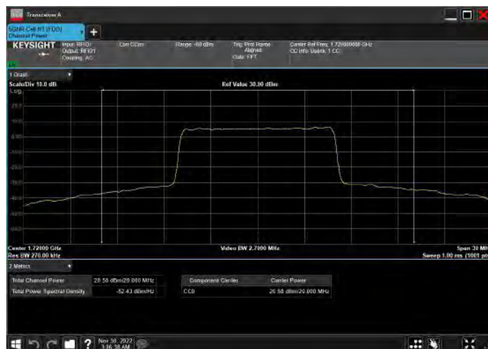
DC_5A_n66A_10MHz|20MHz_15kHz_829MHz|1720MHz_QP SK|CP-OFDM 64 QAM_RB12@0|RB53@26
