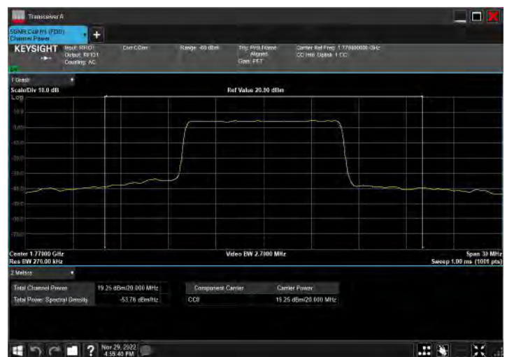
DC_2A_n66A_10MHz|20MHz_15kHz_1905MHz|1770MHz_Q PSK|CP-OFDM 256 QAM_RB12@38|RB53@26
