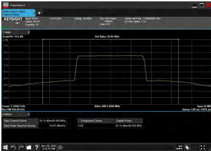
DC_2A_n66A_10MHz|40MHz_15kHz_1880MHz|1745MHz_Q PSK|CP-OFDM QPSK_RB12@0|RB108@54
