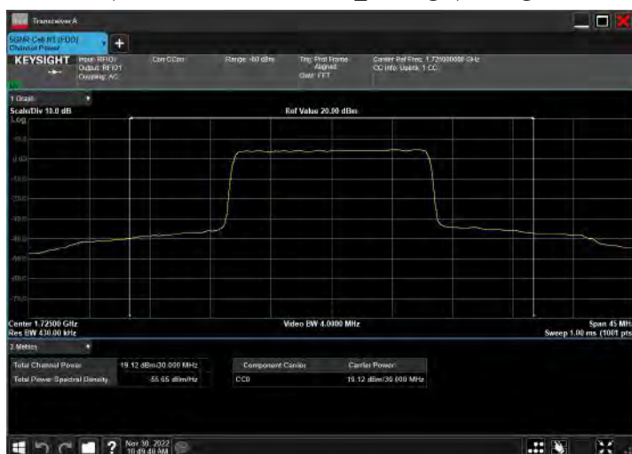
DC_5A_n66A_10MHz|30MHz_15kHz_829MHz|1725MHz_QP SK|DFT-s-OFDM 256 QAM_RB12@0|RB80@40
