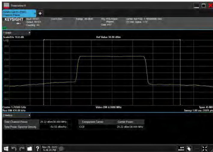
DC_2A_n66A_10MHz|30MHz_15kHz_1905MHz|1765MHz_Q PSK|DFT-s-OFDM 64 QAM_RB12@38|RB80@40
