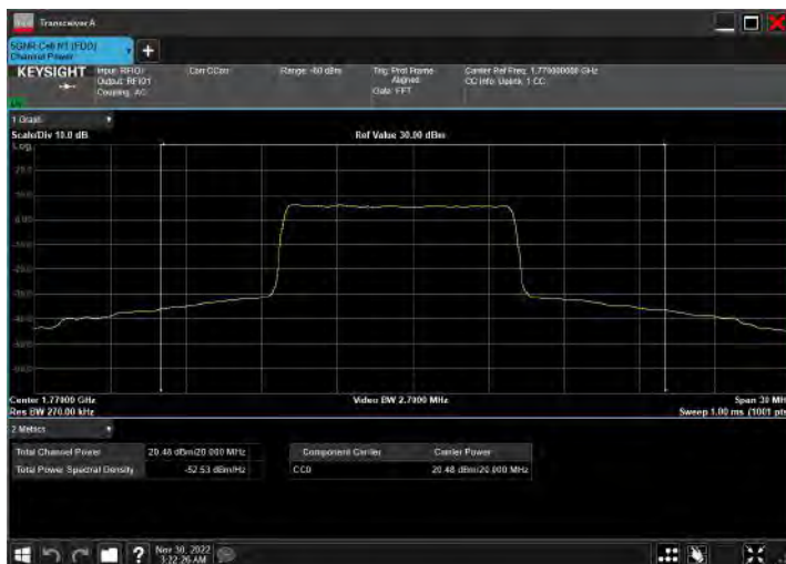
DC_5A_n66A_10MHz|20MHz_15kHz_844MHz|1770MHz_QP SK|DFT-s-OFDM 16 QAM_RB12@38|RB50@25
