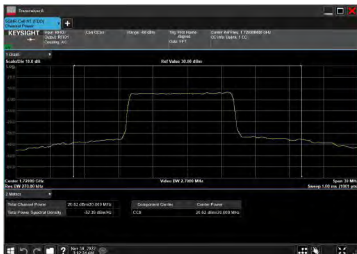
DC_5A_n66A_10MHz|20MHz_15kHz_829MHz|1720MHz_QP SK|DFT-s-OFDM 64 QAM_RB12@0|RB50@25
