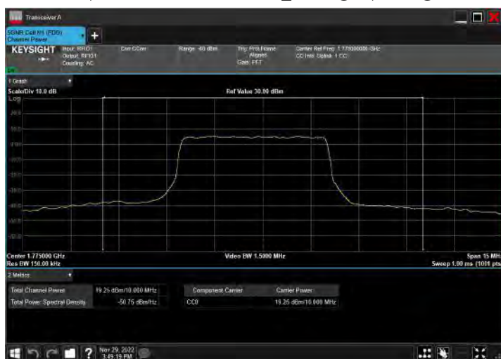
DC_2A_n66A_10MHz|10MHz_15kHz_1905MHz|1775MHz_Q PSK|DFT-s-OFDM 256 QAM_RB12@38|RB25@12
