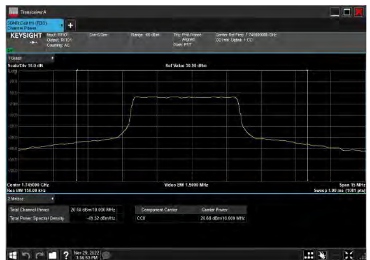
DC_2A_n66A_10MHz|10MHz_15kHz_1880MHz|1745MHz_Q PSK|DFT-s-OFDM 16 QAM_RB12@0|RB25@12
