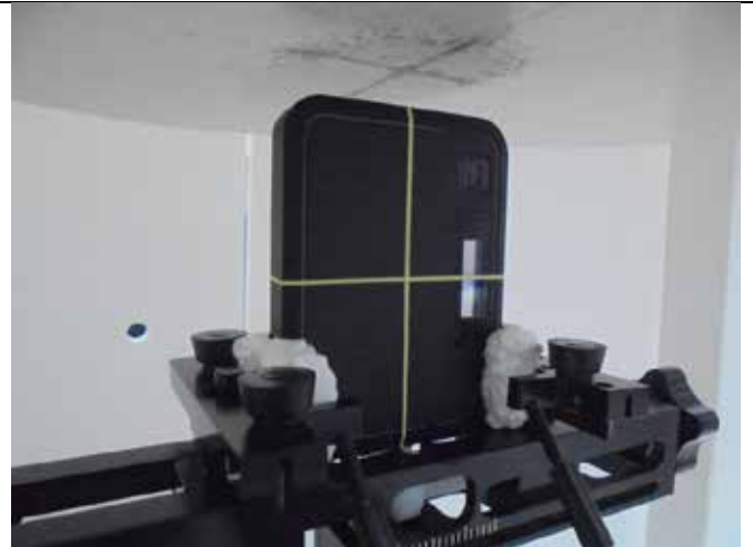
Right Side of EUT with 1.0 cm Gap
