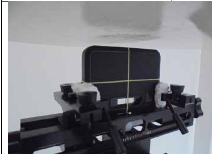
Top Side of EUT with 1.0 cm Gap
