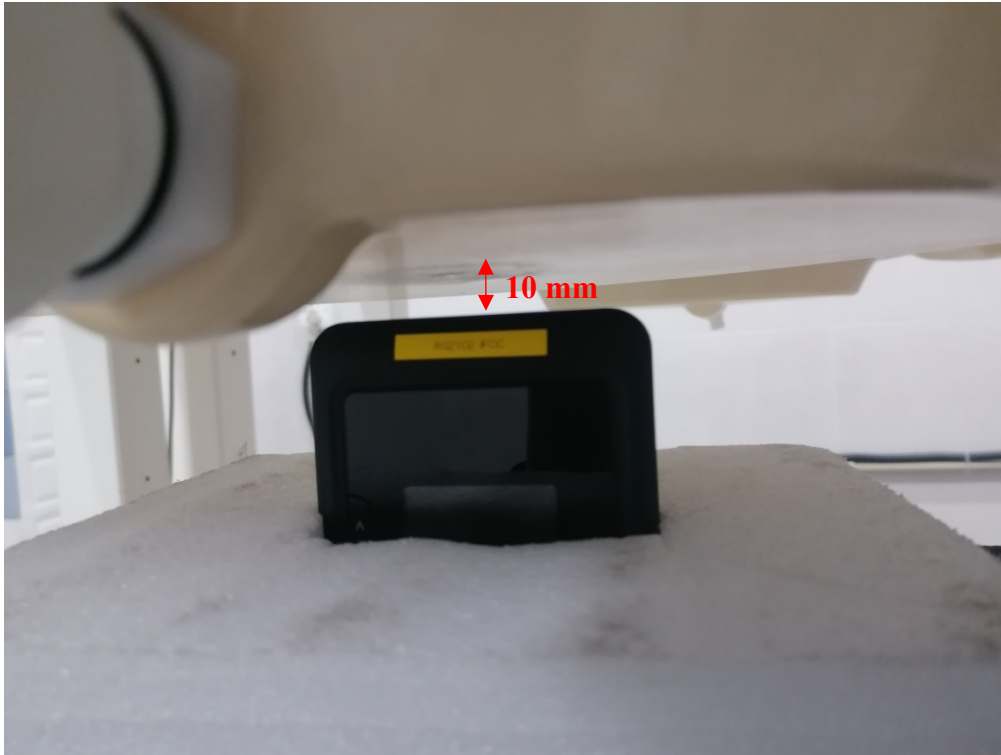
Body Left Setup Photo (10mm)
