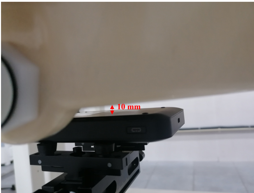
Body (Worn) Back Setup Photo (10mm)
