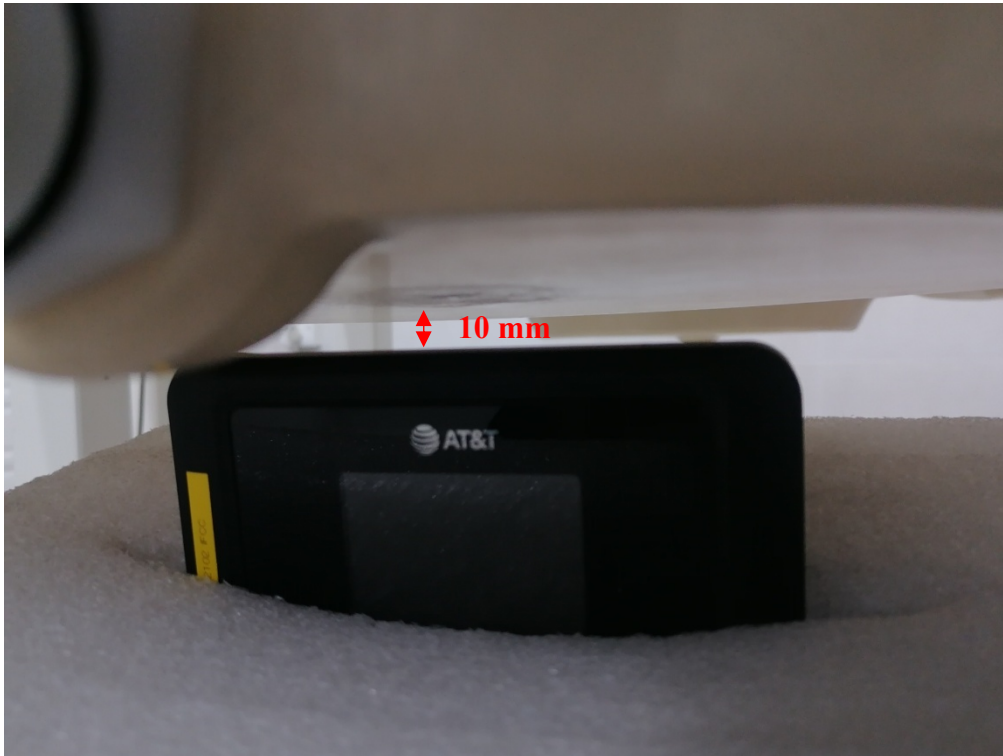
Body Top Setup Photo (10mm)
