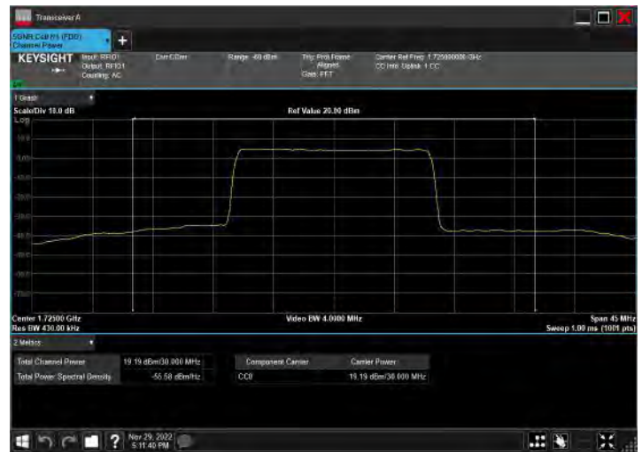
DC_2A_n66A_10MHz|30MHz_15kHz_1855MHz|1725MHz_Q PSK|CP-OFDM 256 QAM_RB12@0|RB80@40
