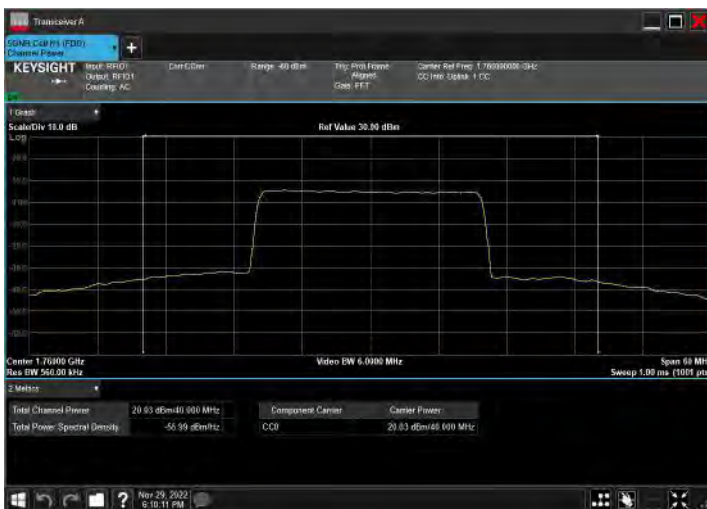
DC_2A_n66A_10MHz|40MHz_15kHz_1905MHz|1760MHz_Q PSK|CP-OFDM 64 QAM_RB12@38|RB108@54
