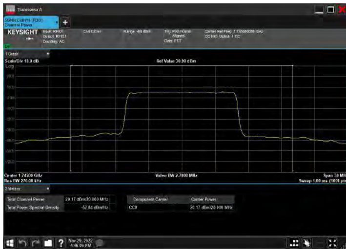
DC_2A_n66A_10MHz|20MHz_15kHz_1880MHz|1745MHz_Q PSK|CP-OFDM 64 QAM_RB12@0|RB53@26
