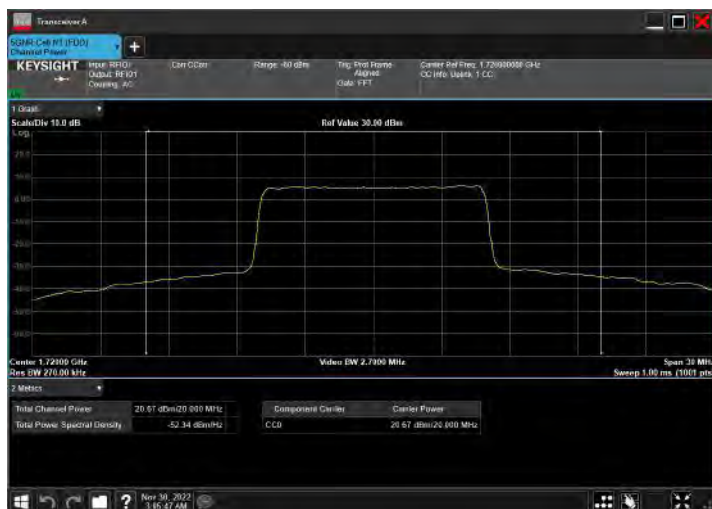
DC_5A_n66A_10MHz|20MHz_15kHz_829MHz|1720MHz_QP SK|CP-OFDM 16 QAM_RB12@0|RB53@26
