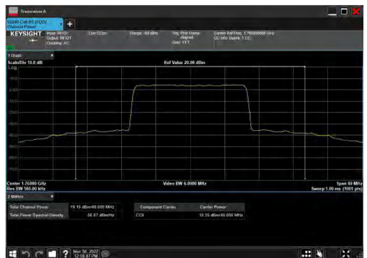
DC_5A_n66A_10MHz|40MHz_15kHz_844MHz|1760MHz_QP SK|CP-OFDM 256 QAM_RB12@38|RB108@54
