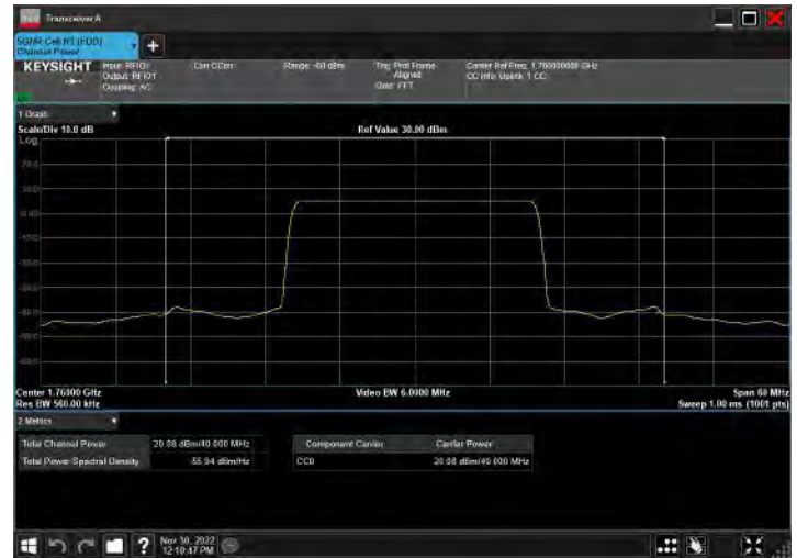
DC_5A_n66A_10MHz|40MHz_15kHz_844MHz|1760MHz_QP SK|DFT-s-OFDM QPSK_RB12@38|RB108@54
