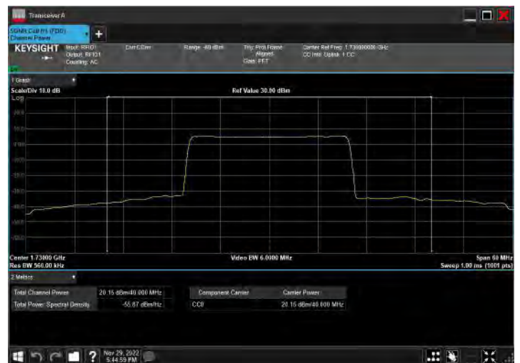
DC_2A_n66A_10MHz|40MHz_15kHz_1855MHz|1730MHz_Q PSK|CP-OFDM QPSK_RB12@0|RB108@54
