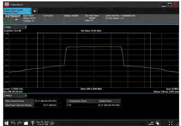
DC_2A_n66A_10MHz|40MHz_15kHz_1880MHz|1745MHz_Q PSK|CP-OFDM 16 QAM_RB12@0|RB108@54
