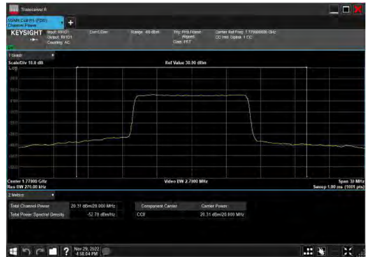
DC_2A_n66A_10MHz|20MHz_15kHz_1905MHz|1770MHz_Q PSK|CP-OFDM 16 QAM_RB12@38|RB53@26
