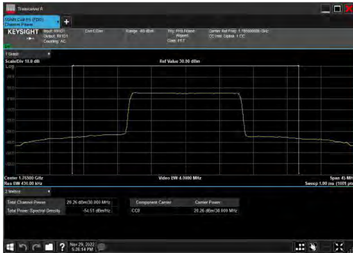
DC_2A_n66A_10MHz|30MHz_15kHz_1905MHz|1765MHz_Q PSK|DFT-s-OFDM 64 QAM_RB12@38|RB80@40
