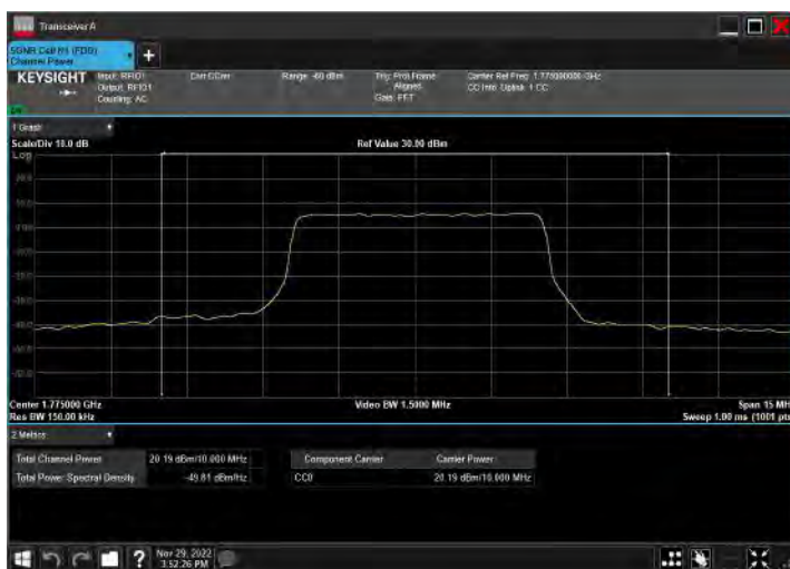
DC_2A_n66A_10MHz|10MHz_15kHz_1905MHz|1775MHz_Q PSK|CP-OFDM 64 QAM_RB12@38|RB26@13
