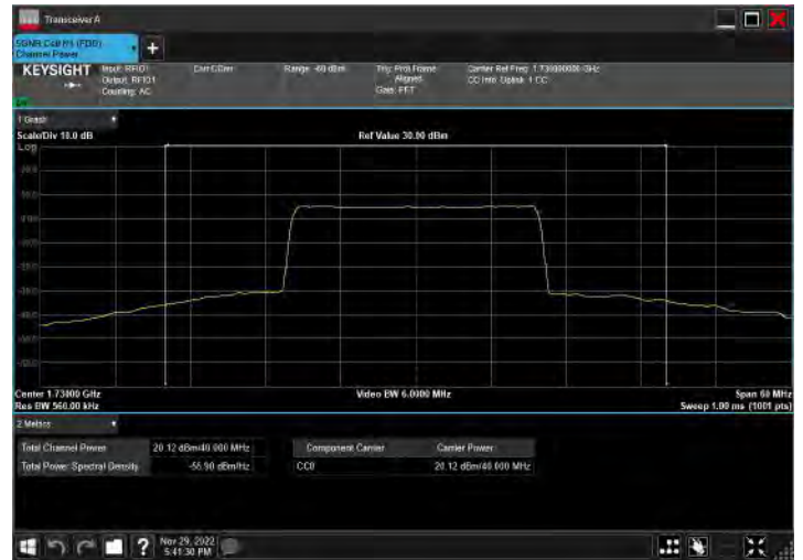
DC_2A_n66A_10MHz|40MHz_15kHz_1855MHz|1730MHz_Q PSK|DFT-s-OFDM 256 QAM_RB12@0|RB108@54
