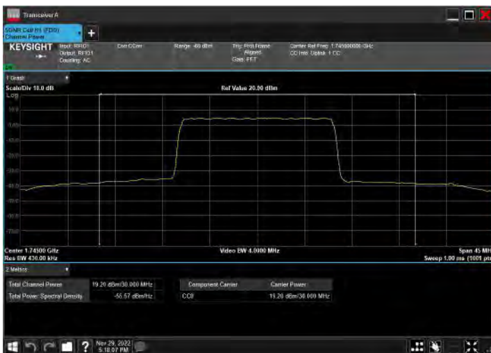
DC_2A_n66A_10MHz|30MHz_15kHz_1880MHz|1745MHz_Q PSK|DFT-s-OFDM 256 QAM_RB12@0|RB80@40
