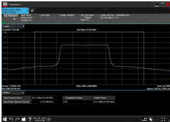
DC_2A_n66A_10MHz|15MHz_15kHz_1880MHz|1745MHz_Q PSK|DFT-s-OFDM 16 QAM_RB12@0|RB36@18
