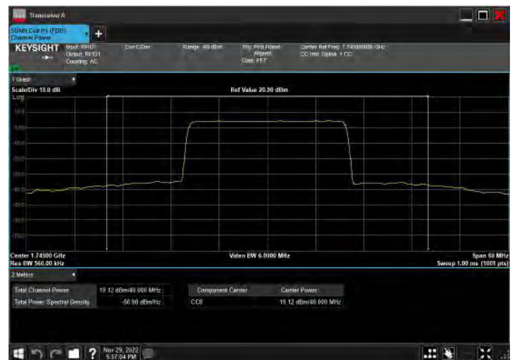
DC_2A_n66A_10MHz|40MHz_15kHz_1880MHz|1745MHz_Q PSK|CP-OFDM 256 QAM_RB12@0|RB108@54
