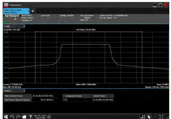
DC_2A_n66A_10MHz|10MHz_15kHz_1905MHz|1775MHz_Q PSK|DFT-s-OFDM 64 QAM_RB12@38|RB25@12
