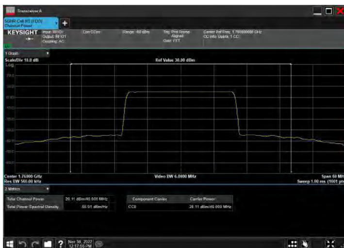
DC_5A_n66A_10MHz|40MHz_15kHz_844MHz|1760MHz_QP SK|CP-OFDM 64 QAM_RB12@38|RB108@54
