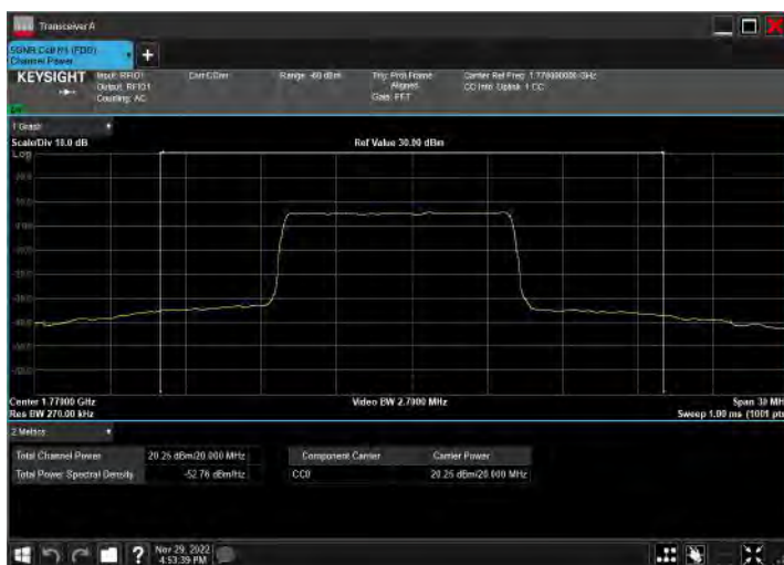
DC_2A_n66A_10MHz|20MHz_15kHz_1905MHz|1770MHz_Q PSK|DFT-s-OFDM 16 QAM_RB12@38|RB50@25
