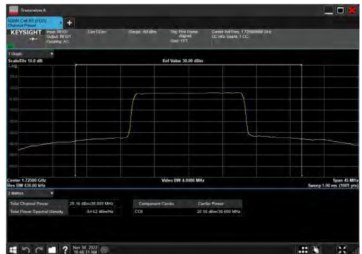
DC_5A_n66A_10MHz|30MHz_15kHz_829MHz|1725MHz_QP SK|DFT-s-OFDM 64 QAM_RB12@0|RB80@40
