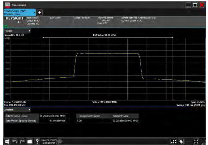
DC_2A_n66A_10MHz|30MHz_15kHz_1905MHz|1765MHz_Q PSK|DFT-s-OFDM 256 QAM_RB12@38|RB80@40
