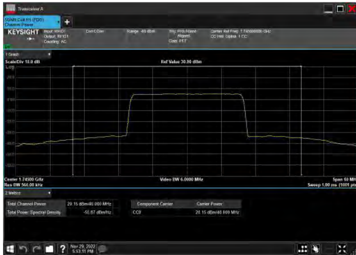
DC_2A_n66A_10MHz|40MHz_15kHz_1880MHz|1745MHz_Q PSK|CP-OFDM QPSK_RB12@0|RB108@54
