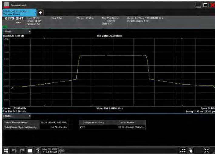
DC_5A_n66A_10MHz|40MHz_15kHz_829MHz|1730MHz_QP SK|DFT-s-OFDM 64 QAM_RB12@0|RB108@54
