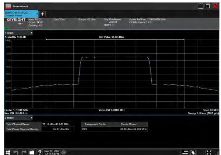
DC_5A_n66A_10MHz|40MHz_15kHz_844MHz|1760MHz_QP SK|DFT-s-OFDM 64 QAM_RB12@38|RB108@54
