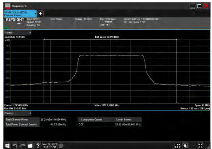
DC_2A_n66A_10MHz|10MHz_15kHz_1905MHz|1775MHz_Q PSK|CP-OFDM 16 QAM_RB12@38|RB26@13
