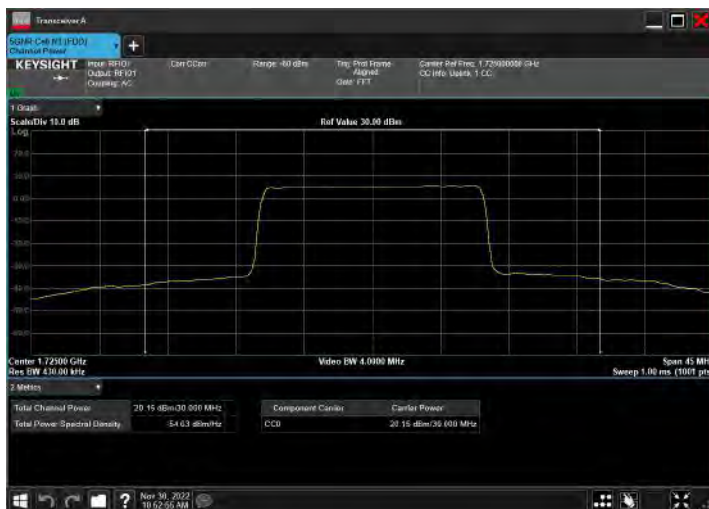
DC_5A_n66A_10MHz|30MHz_15kHz_829MHz|1725MHz_QP SK|CP-OFDM 64 QAM_RB12@0|RB80@40
