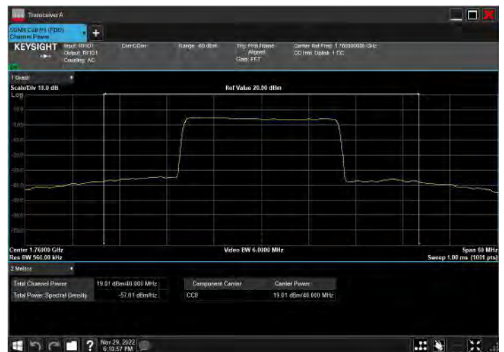
DC_2A_n66A_10MHz|40MHz_15kHz_1905MHz|1760MHz_Q PSK|CP-OFDM 256 QAM_RB12@38|RB108@54
