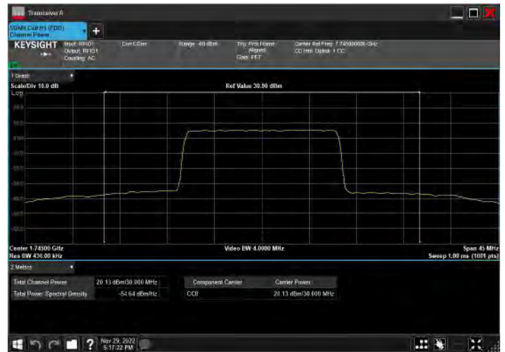
DC_2A_n66A_10MHz|30MHz_15kHz_1880MHz|1745MHz_Q PSK|DFT-s-OFDM 64 QAM_RB12@0|RB80@40
