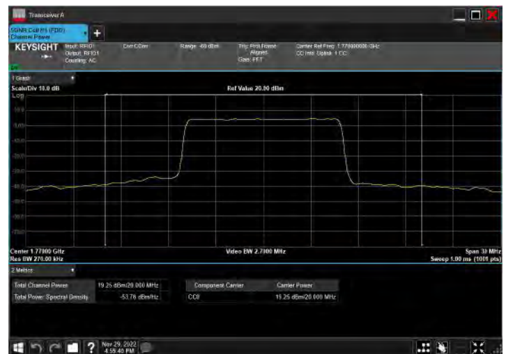
DC_2A_n66A_10MHz|20MHz_15kHz_1905MHz|1770MHz_Q PSK|CP-OFDM 256 QAM_RB12@38|RB53@26
