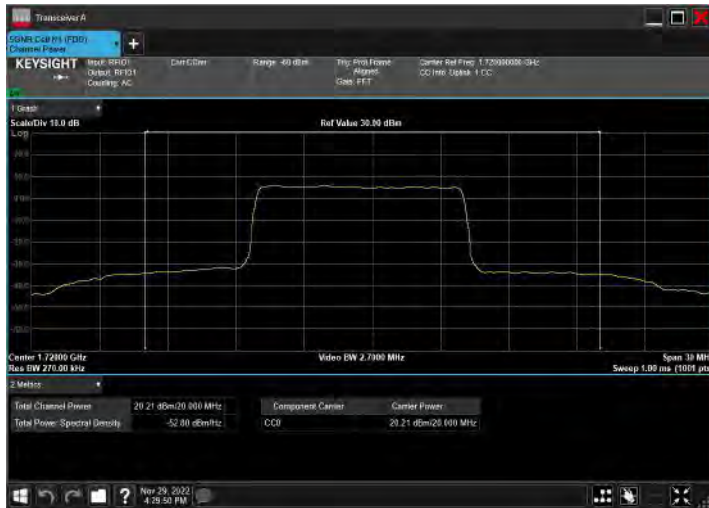
DC_2A_n66A_10MHz|20MHz_15kHz_1855MHz|1720MHz_Q PSK|DFT-s-OFDM 64 QAM_RB12@0|RB50@25
