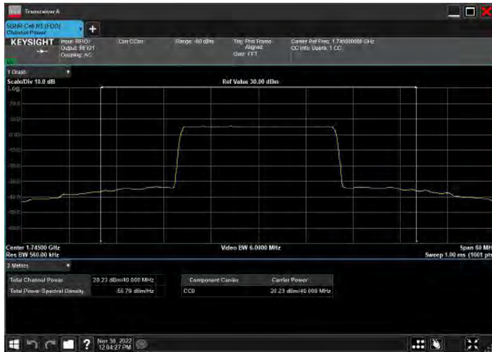
DC_5A_n66A_10MHz|40MHz_15kHz_836.5MHz|1745MHz_Q PSK|CP-OFDM QPSK_RB12@0|RB108@54
