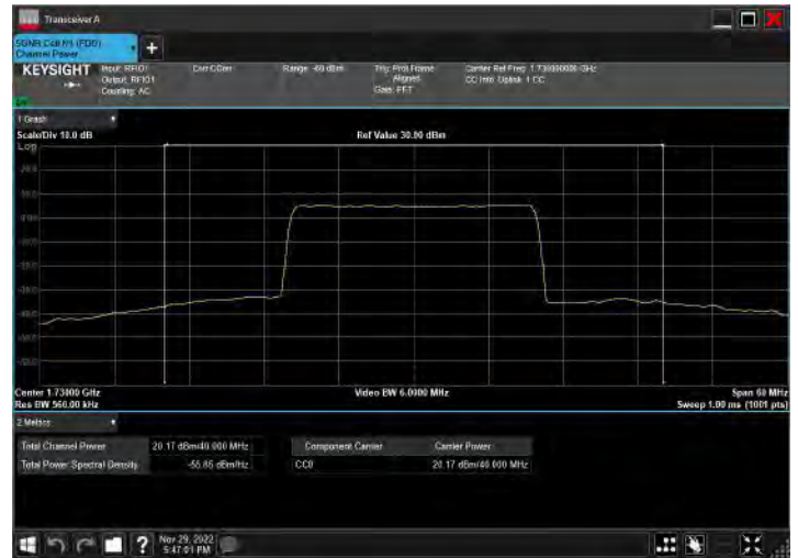
DC_2A_n66A_10MHz|40MHz_15kHz_1880MHz|1745MHz_Q PSK|DFT-s-OFDM PI/2 BPSK_RB12@0|RB108@54
