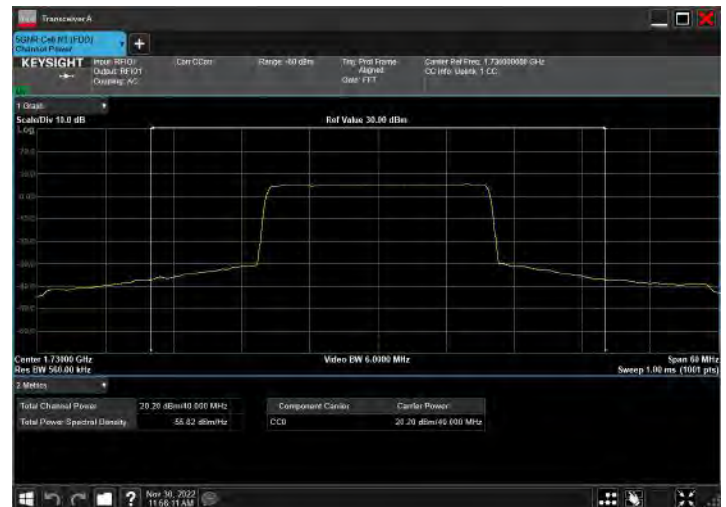
DC_5A_n66A_10MHz|40MHz_15kHz_829MHz|1730MHz_QP SK|CP-OFDM QPSK_RB12@0|RB108@54
