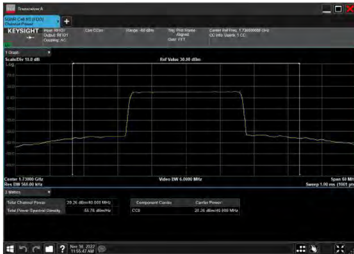
DC_5A_n66A_10MHz|40MHz_15kHz_829MHz|1730MHz_QP SK|DFT-s-OFDM 64 QAM_RB12@0|RB108@54
