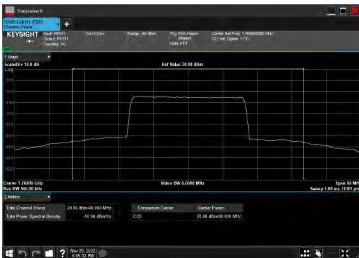
DC_2A_n66A_10MHz|40MHz_15kHz_1905MHz|1760MHz_Q PSK|DFT-s-OFDM 16 QAM_RB12@38|RB108@54
