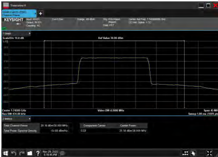
DC_2A_n66A_10MHz|30MHz_15kHz_1880MHz|1745MHz_Q PSK|CP-OFDM 256 QAM_RB12@0|RB80@40
