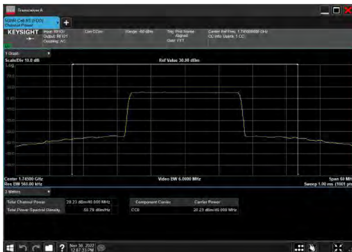
DC_5A_n66A_10MHz|40MHz_15kHz_836.5MHz|1745MHz_Q PSK|CP-OFDM 64 QAM_RB12@0|RB108@54
