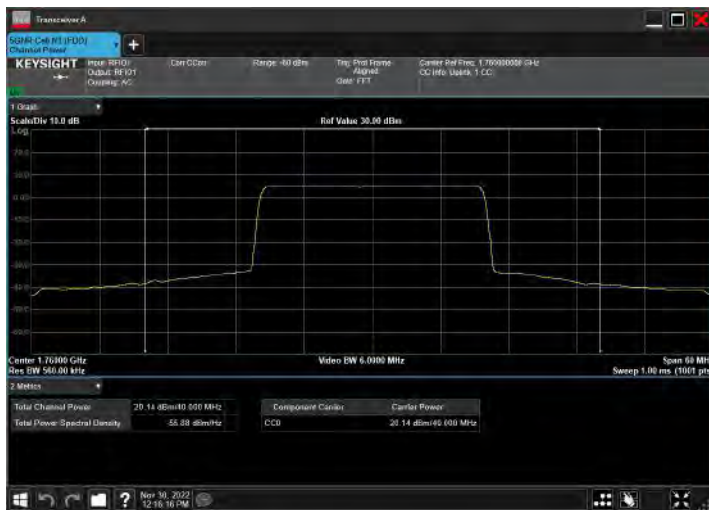
DC_5A_n66A_10MHz|40MHz_15kHz_844MHz|1760MHz_QP SK|CP-OFDM QPSK_RB12@38|RB108@54
