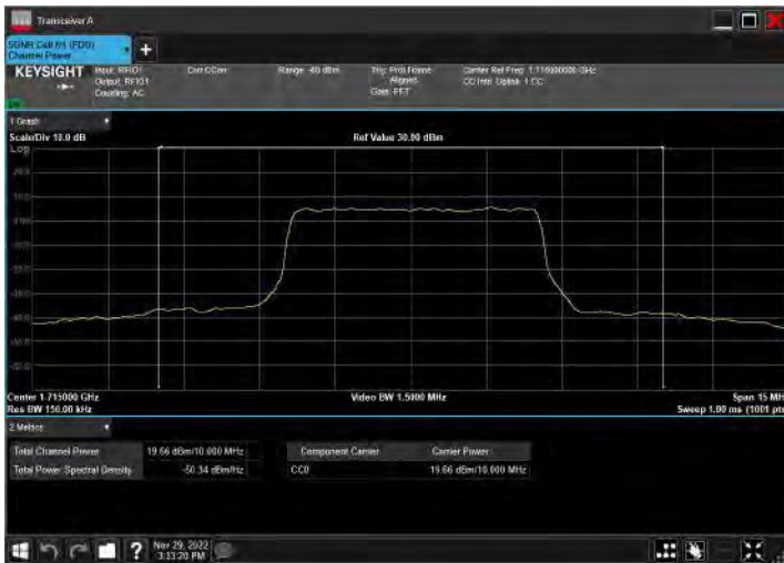
DC_2A_n66A_10MHz|10MHz_15kHz_1855MHz|1715MHz_Q PSK|CP-OFDM 256 QAM_RB12@0|RB26@13
