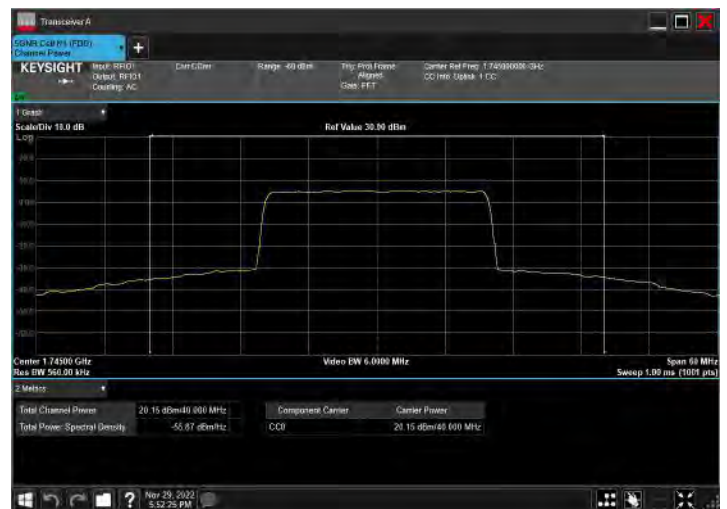
DC_2A_n66A_10MHz|40MHz_15kHz_1880MHz|1745MHz_Q PSK|DFT-s-OFDM 16 QAM_RB12@0|RB108@54
