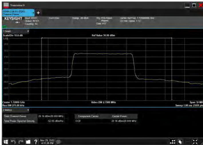
DC_2A_n66A_10MHz|20MHz_15kHz_1855MHz|1720MHz_Q PSK|DFT-s-OFDM 64 QAM_RB12@0|RB50@25
