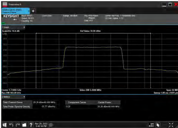
DC_2A_n66A_10MHz|40MHz_15kHz_1855MHz|1730MHz_Q PSK|DFT-s-OFDM 64 QAM_RB12@0|RB108@54
