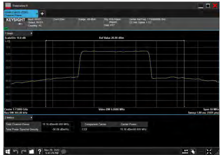
DC_2A_n66A_10MHz|40MHz_15kHz_1855MHz|1730MHz_Q PSK|DFT-s-OFDM 256 QAM_RB12@0|RB108@54
