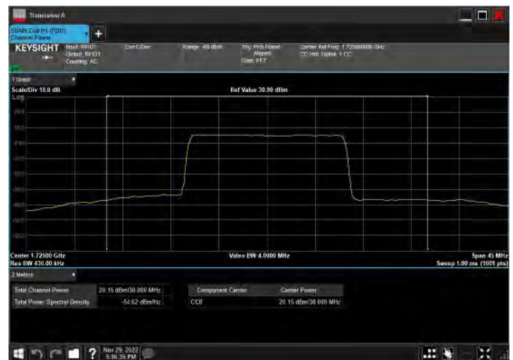
DC_2A_n66A_10MHz|30MHz_15kHz_1855MHz|1725MHz_Q PSK|DFT-s-OFDM 64 QAM_RB12@0|RB80@40
