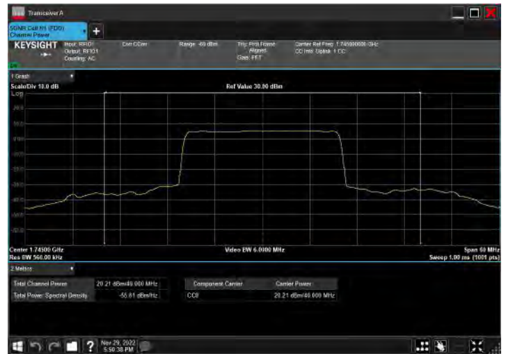
DC_2A_n66A_10MHz|40MHz_15kHz_1880MHz|1745MHz_Q PSK|DFT-s-OFDM PI/2 BPSK_RB12@0|RB108@54
