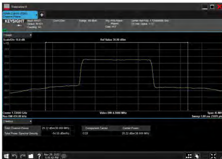
DC_2A_n66A_10MHz|30MHz_15kHz_1855MHz|1725MHz_Q PSK|DFT-s-OFDM 16 QAM_RB12@0|RB80@40
