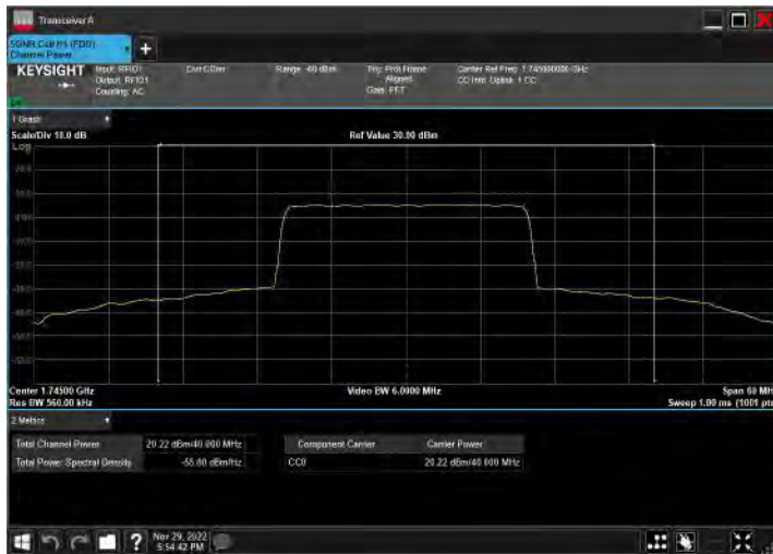
DC_2A_n66A_10MHz|40MHz_15kHz_1880MHz|1745MHz_Q PSK|CP-OFDM QPSK_RB12@0|RB108@54
