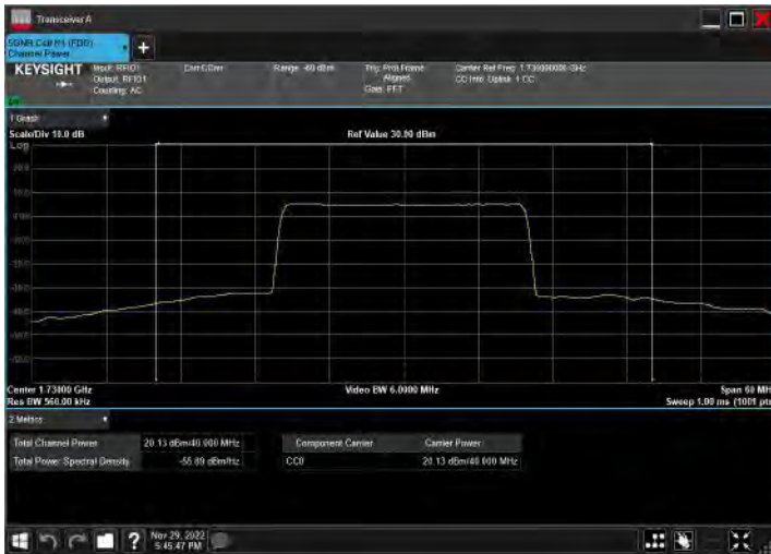
DC_2A_n66A_10MHz|40MHz_15kHz_1855MHz|1730MHz_Q PSK|CP-OFDM 256 QAM_RB12@0|RB108@54
