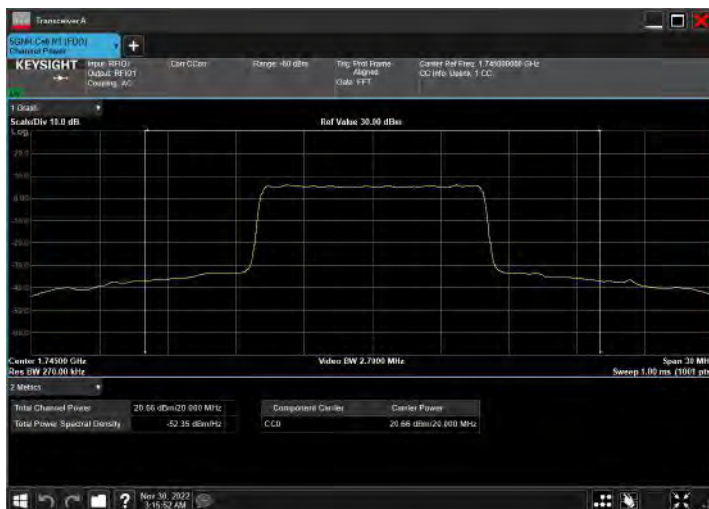
DC_5A_n66A_10MHz|20MHz_15kHz_836.5MHz|1745MHz_Q PSK|CP-OFDM 64 QAM_RB12@0|RB53@26
