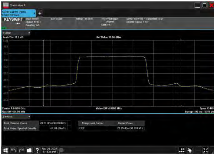
DC_2A_n66A_10MHz|30MHz_15kHz_1880MHz|1745MHz_Q PSK|DFT-s-OFDM 16 QAM_RB12@0|RB80@40
