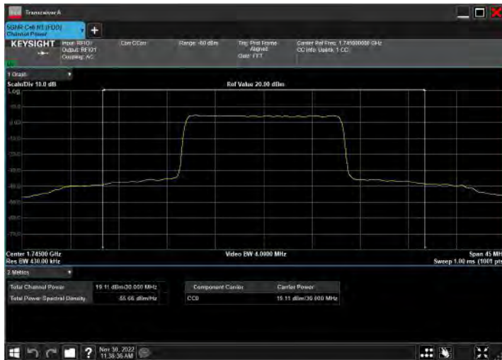
DC_5A_n66A_10MHz|30MHz_15kHz_836.5MHz|1745MHz_Q PSK|CP-OFDM 256 QAM_RB12@0|RB80@40
