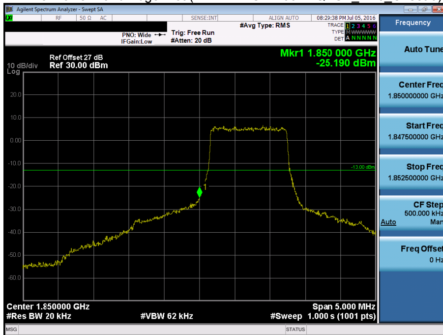
BAND 25. Lower Band Edge Plot (1.4M BW Ch. 26047 QPSK_RB6_Offset 0) -2
