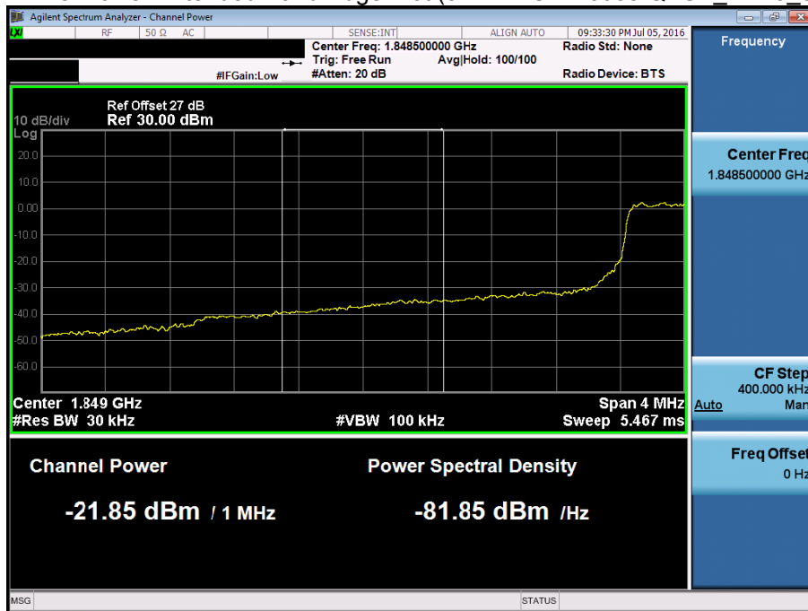
BAND 25. Lower Extended Band Edge Plot (3M BW Ch. 26055 QPSK_RB15_0) -3
