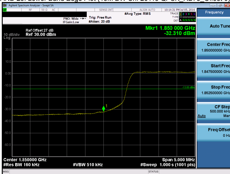
BAND 25. Lower Band Edge Plot (15M BW Ch. 26115 QPSK_RB75_Offset 0) -2
