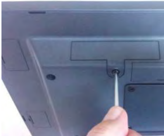
HDD access panel
