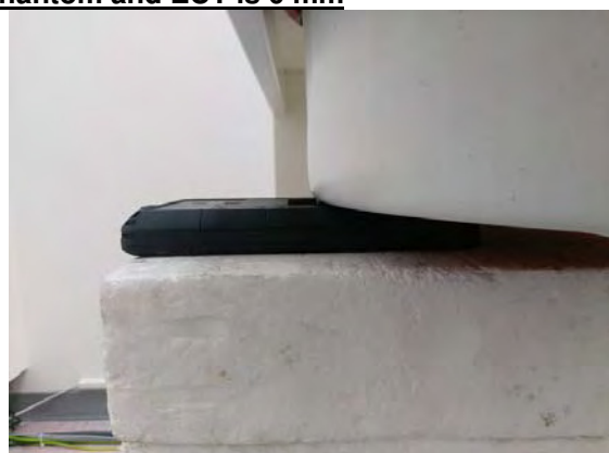
Fig.3 EUT Back side (Main) to flat phantom
