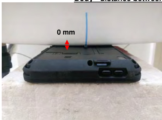
Fig.3 EUT Back side (Main) to flat phantom
