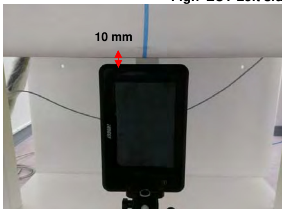
Fig.8 EUT Left side (10mm) to flat phantom
