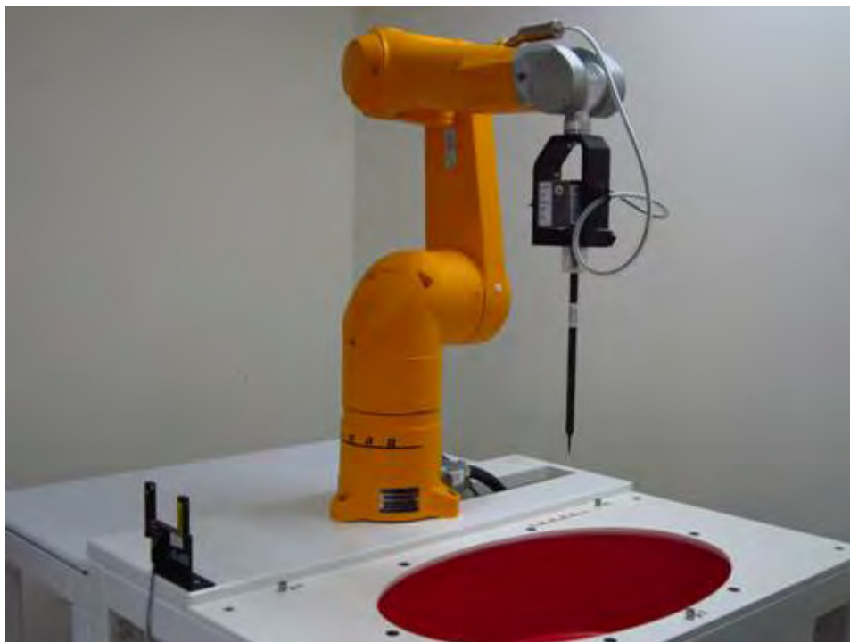
Fig.1 Photograph of the SAR measurement system
