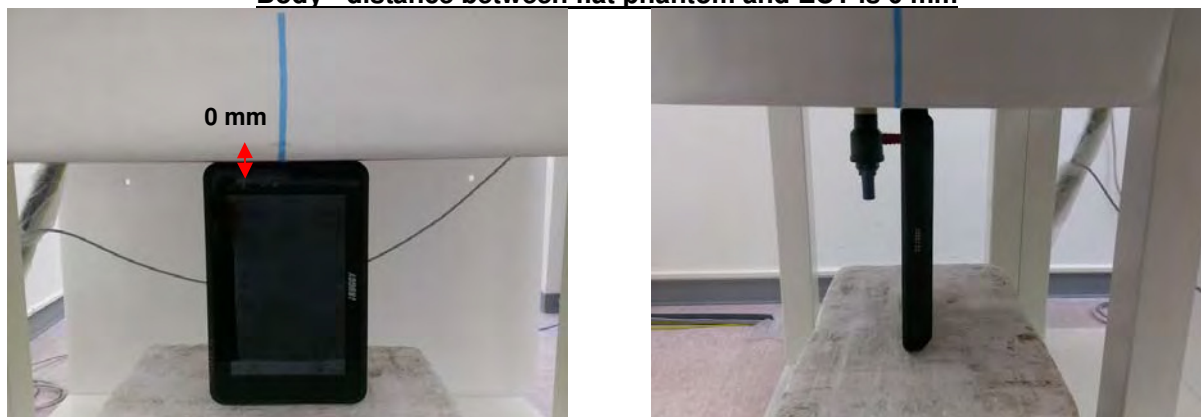
Fig.9 EUT Right side to flat phantom
