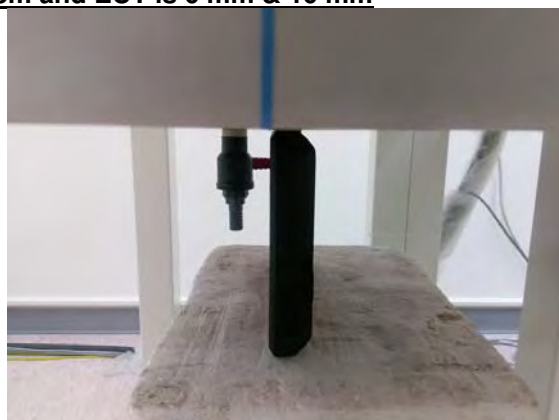
Fig.6 EUT Bottom side to flat phantom
