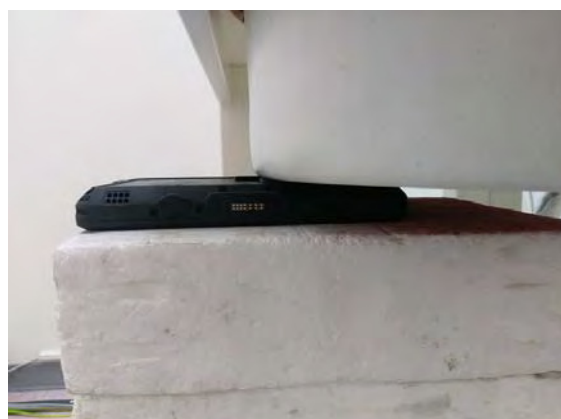
Fig.4 EUT Back side (Aux) to flat phantom
