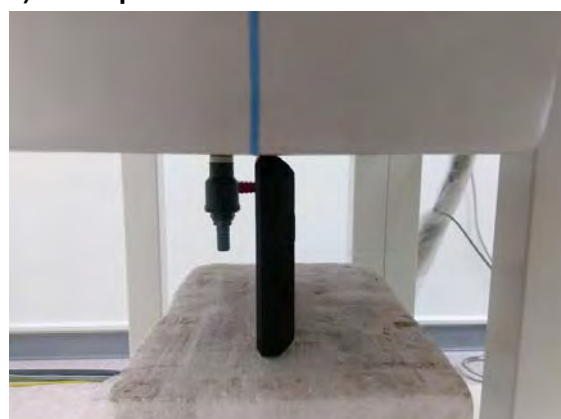
Fig.5 EUT Top side to flat phantom
