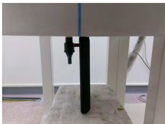
Fig.7 EUT Left side (0mm) to flat phantom
