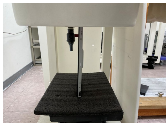
Fig.5 EUT Right side to flat phantom
