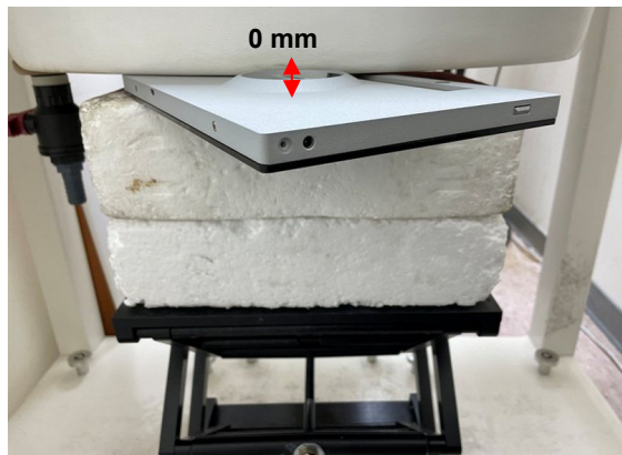
Fig.3 EUT Back side to flat phantom
