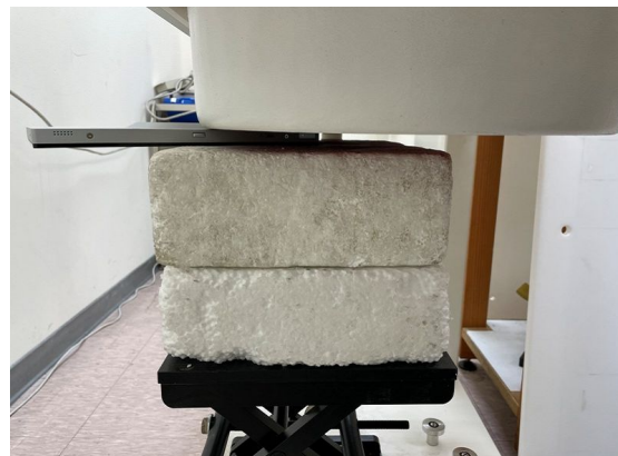
Fig.3 EUT Back side to flat phantom
