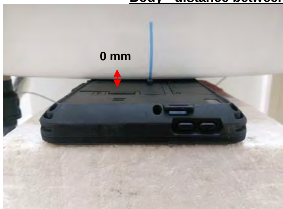
Fig.3 EUT Back side (Main) to flat phantom
