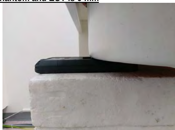
Fig.3 EUT Back side (Main) to flat phantom
