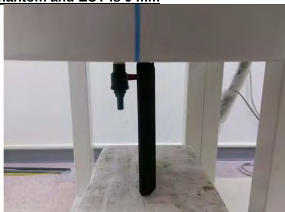
Fig.6 EUT Left side to flat phantom
