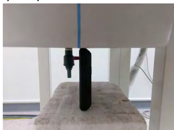
Fig.5 EUT Top side to flat phantom
