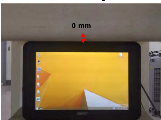
Fig.5 EUT Top side to flat phantom
