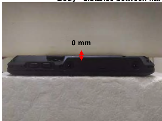
Fig.3 EUT Back side to flat phantom
