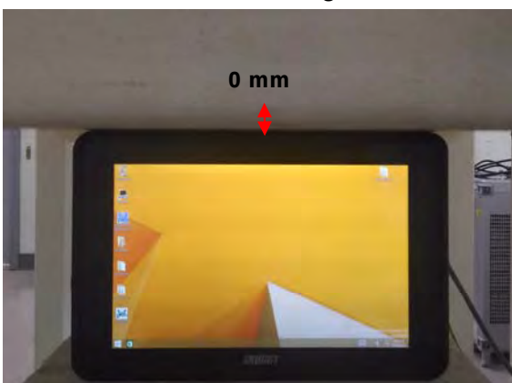
Fig.5 EUT Top side to flat phantom
