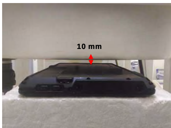
Fig.4 EUT Back side (10mm) to flat phantom
