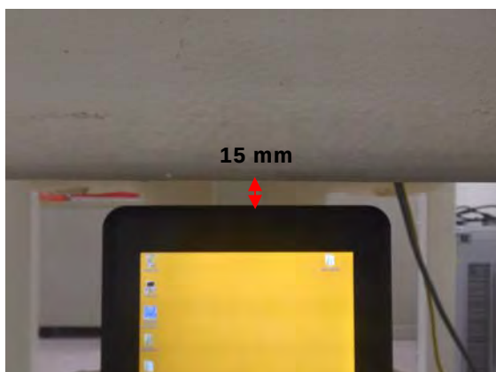
Fig.7 EUT Left side (15mm) to flat phantom
