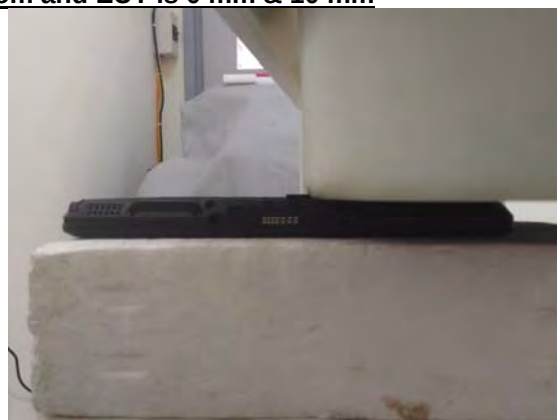
Fig.3 EUT Back side to flat phantom
