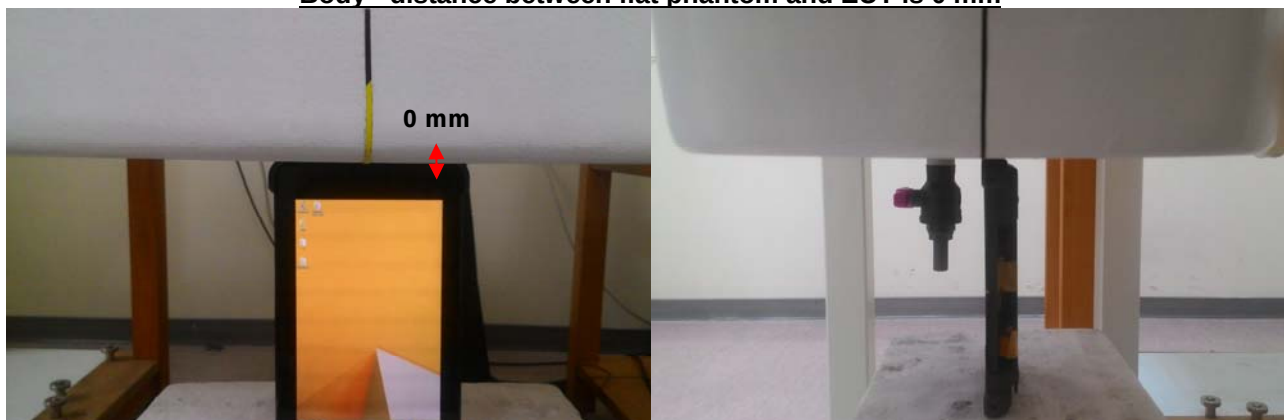
Fig.6 EUT Left side to flat phantom
