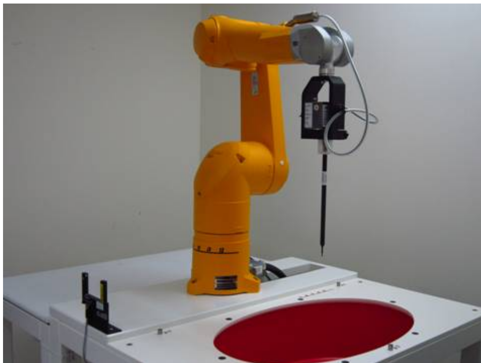
Fig.1 Photograph of the SAR measurement system
