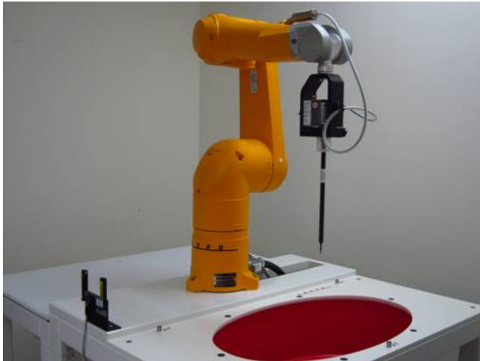
Fig.1 Photograph of the SAR measurement system
