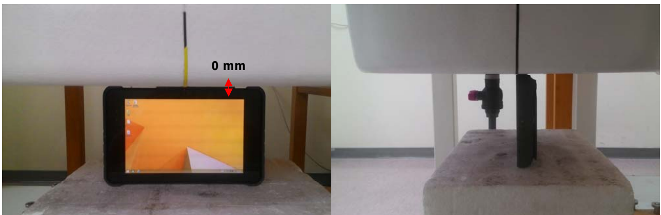
Fig.4 EUT Top side to flat phantom
