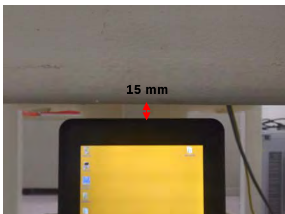
Fig.8 EUT Left side (15mm) to flat phantom
