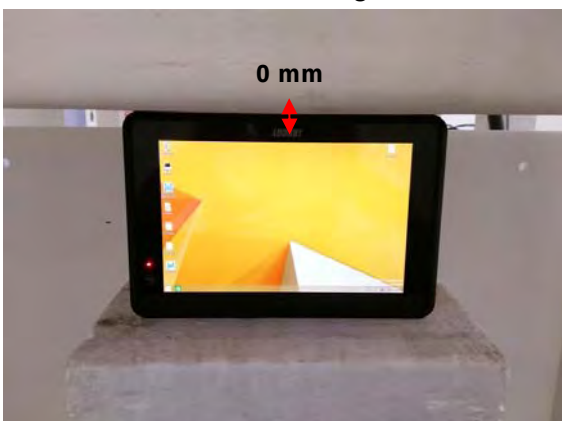
Fig.5 EUT Bottom side to flat phantom
