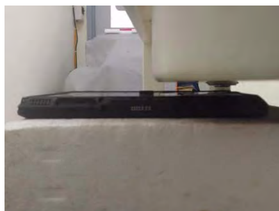
Fig.4 EUT Back side (10mm) to flat phantom
