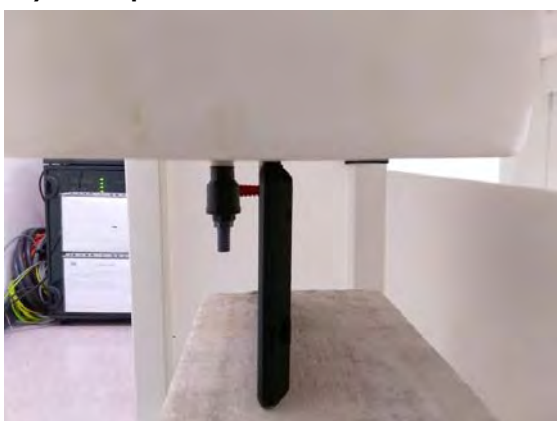
Fig.5 EUT Bottom side to flat phantom
