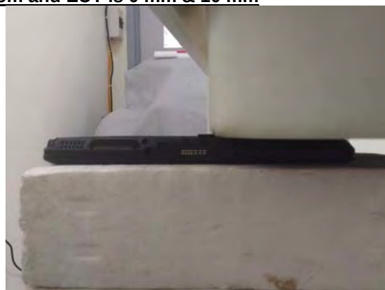
Fig.3 EUT Back side to flat phantom
