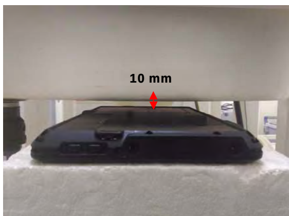
Fig.4 EUT Back side (10mm) to flat phantom
