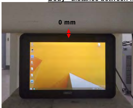
Fig.6 EUT Top side to flat phantom
