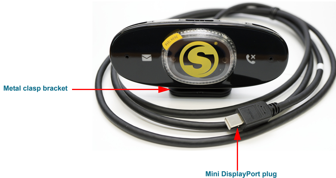
Back view of Remote Camera Unit
