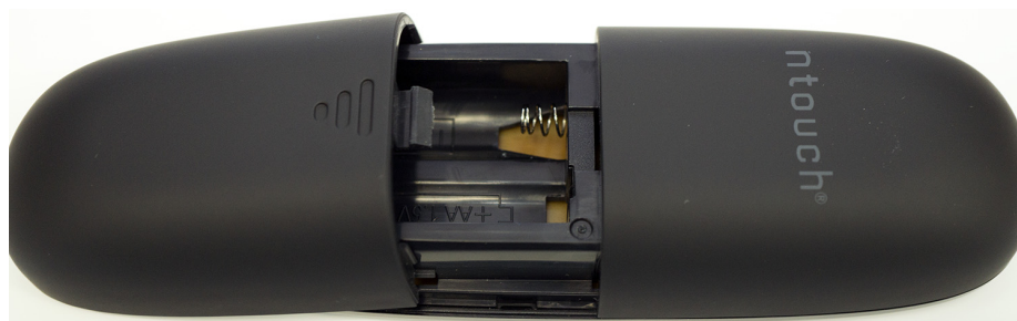
Back view of Remote Control Unit showing open battery compartment
