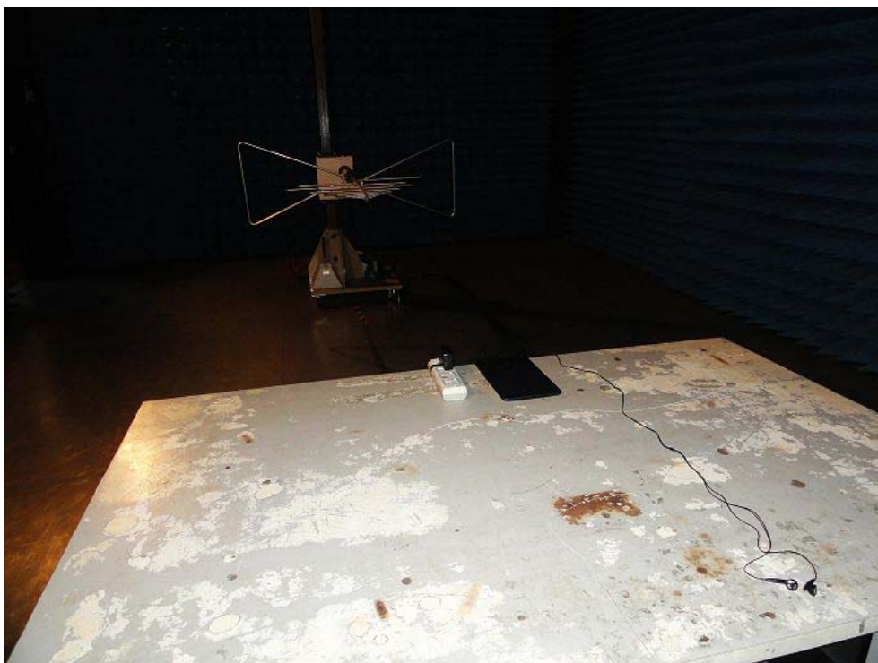
Radiated Emission Test Setup:
