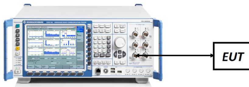
Figure 7-7. ERP/EIRP Measurement Setup
