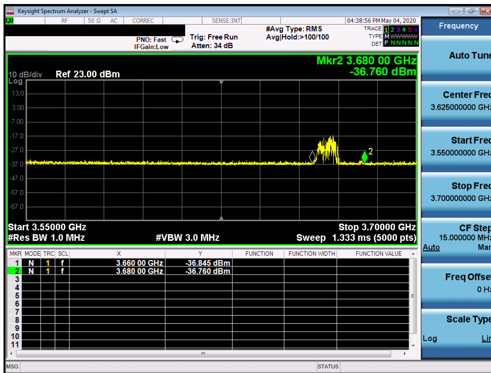
Plot 20. Conducted Measurement - UUT RF transmission range and bandwidths are less or equal to frequency range and bandwidth of compatible BTS-CBSD (WINNF.FT.C.DRG.1)
