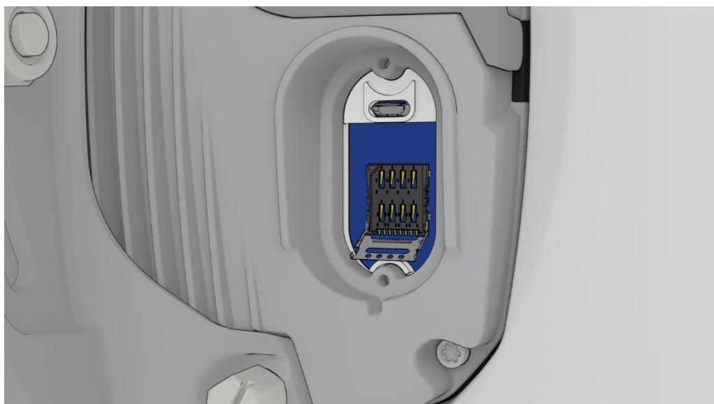
Figure 4 - Opening the SIM locking mechanism
