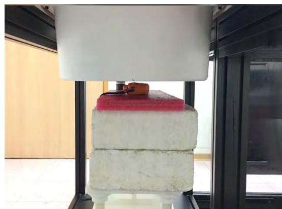
Fig.4 EUT Right side to flat phantom
