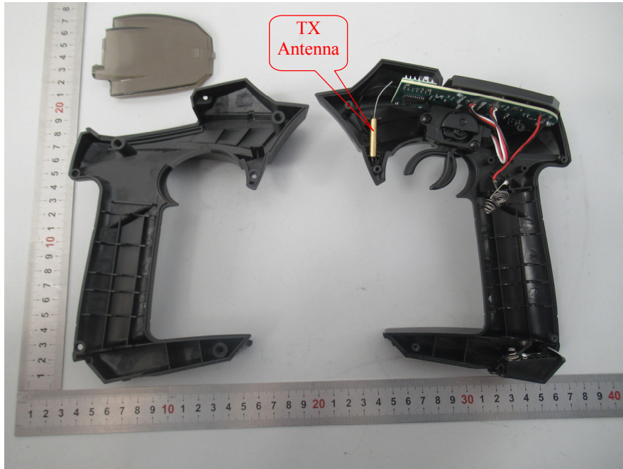
EUT – Cover off View-2 (MT-203)
