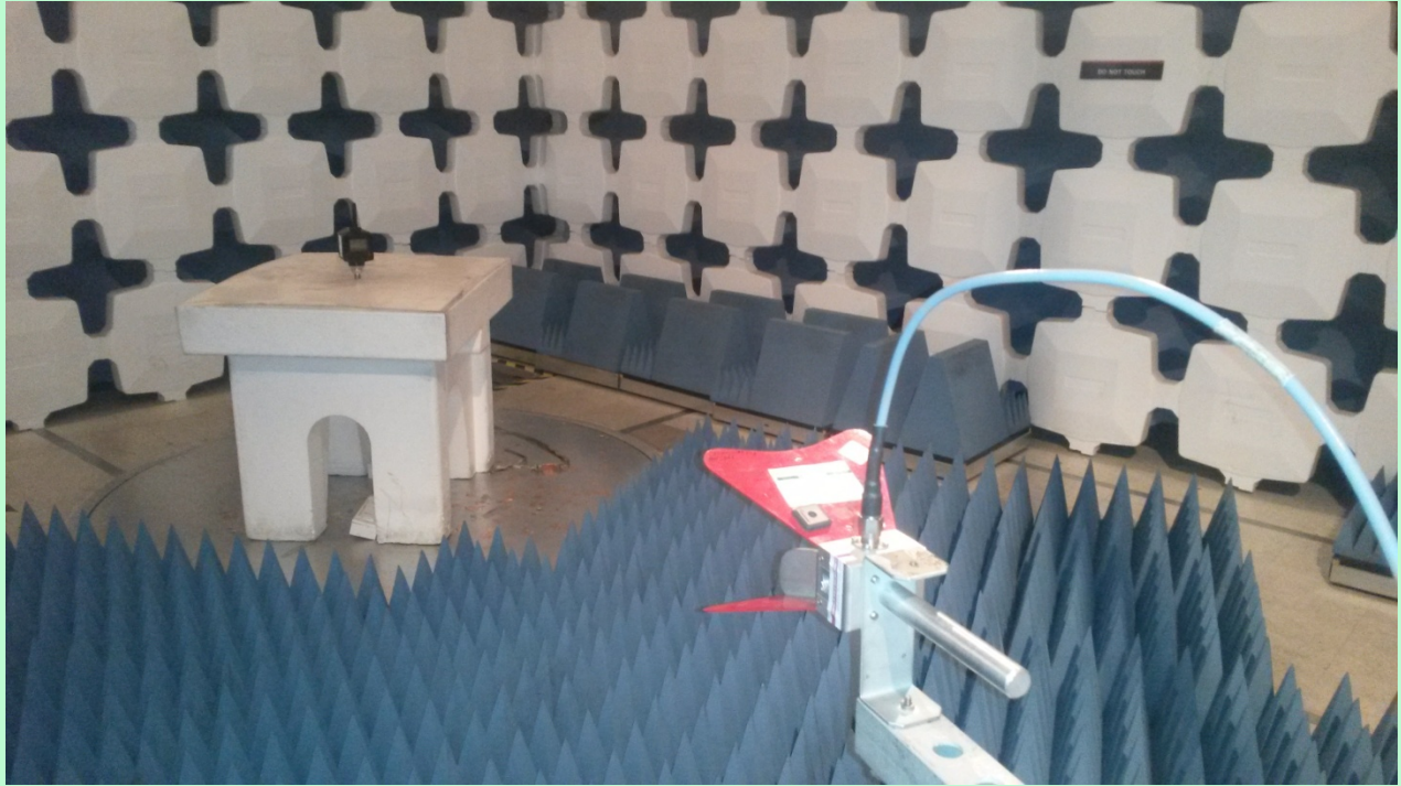
Test Setup : Transmitter Output Power and Dwell Time
