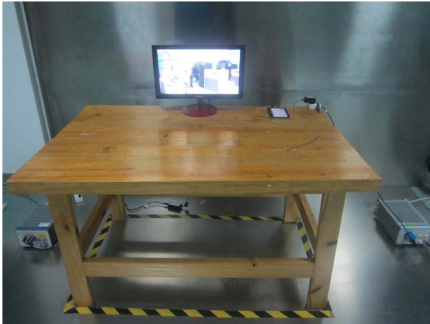
Conducted Emissions – Side View
