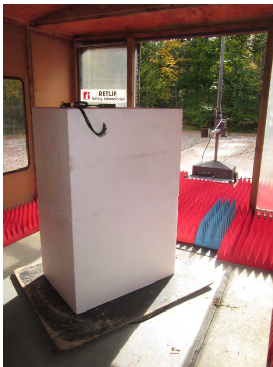
Horizontal Antenna Polarization, 12 GHz to 18 GHz, Internal Antenna, 150 cm
