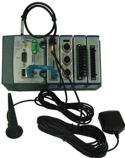
Fig. 1: Wiring of cRIO GXXX 3G Mobile Module
