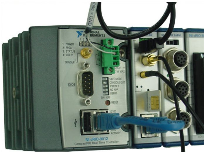
Fig. 3: Wiring the cRIO Gxxx 3G Mobile Module - Details
