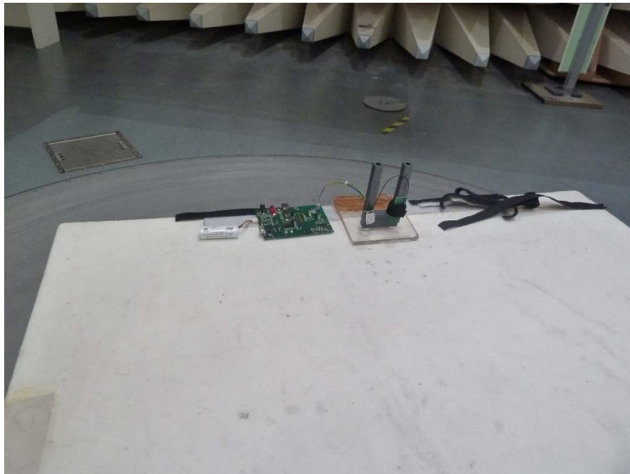
Photo 24: EUT with external PCB antenna in the semi-anechoic chamber
