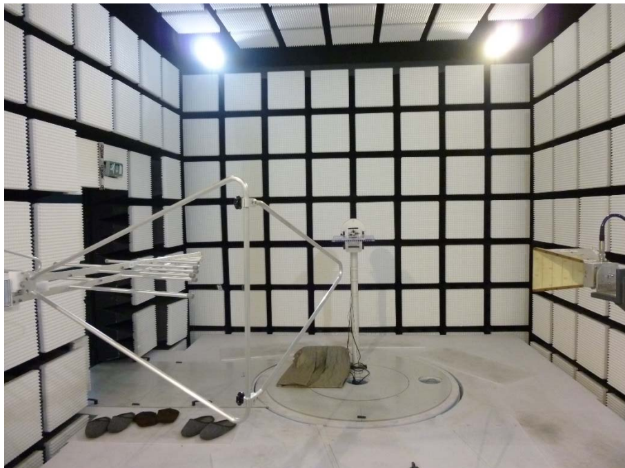
Photo 6: EUT with internal antenna in the anechoic chamber
