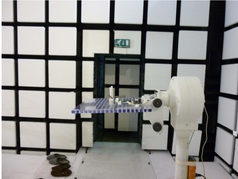
Photo 19: EUT with external PCB antenna in the anechoic chamber
