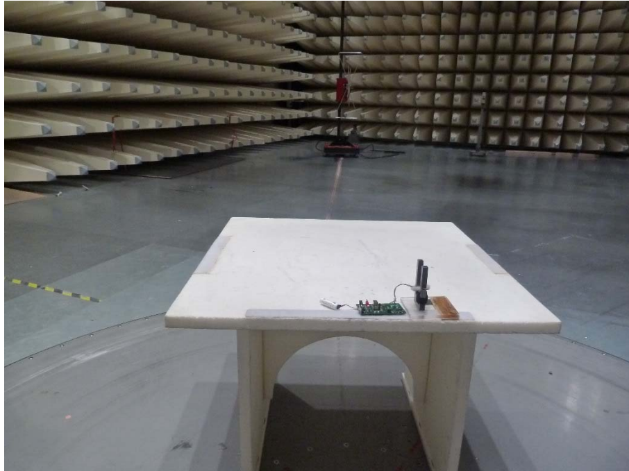
Photo 7: EUT with internal antenna in the semi-anechoic chamber
