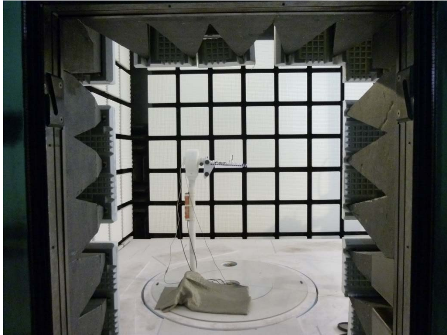
Photo 9: EUT with external rubber antenna in the anechoic chamber
