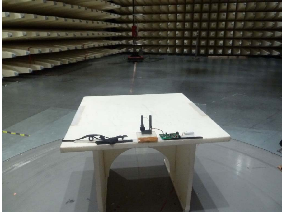
Photo 23: EUT with external PCB antenna in the semi-anechoic chamber
