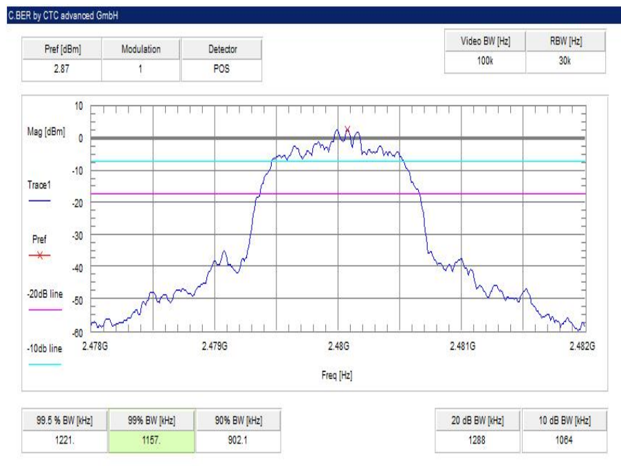
Plot 6: highest channel – 2480 MHz, Pi / DQPSK modulation
