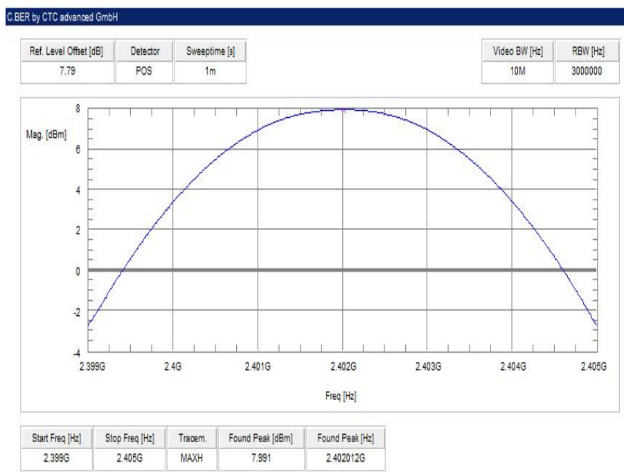
Plot 1: lowest channel – 2402 MHz, GFSK modulation
