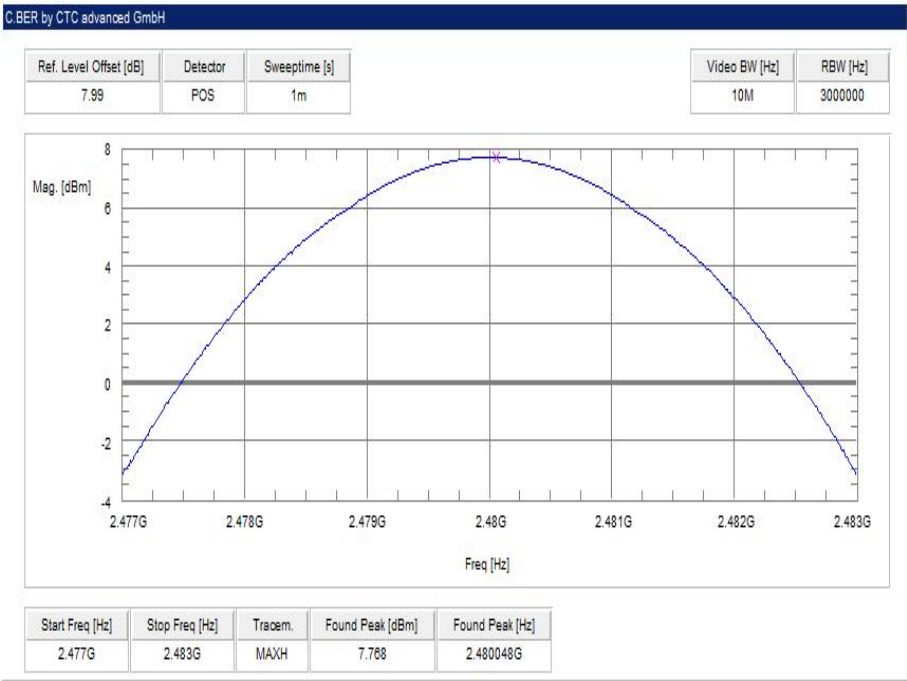
Plot 9: highest channel – 2480 MHz, 8 DPSK modulation
