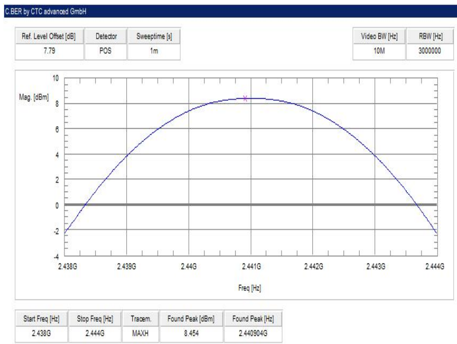
Plot 2: middle channel – 2441 MHz, GFSK modulation
