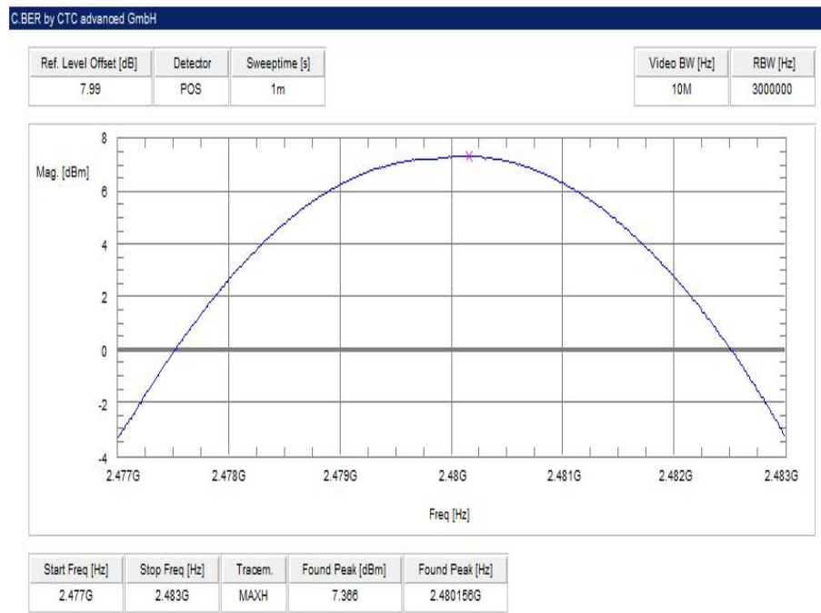
Plot 6: highest channel – 2480 MHz, Pi / DQPSK modulation
