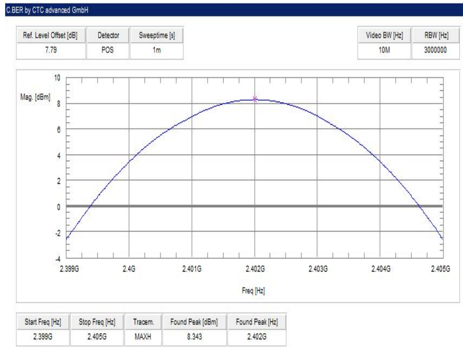
Plot 7: lowest channel – 2402 MHz, 8 DPSK modulation
