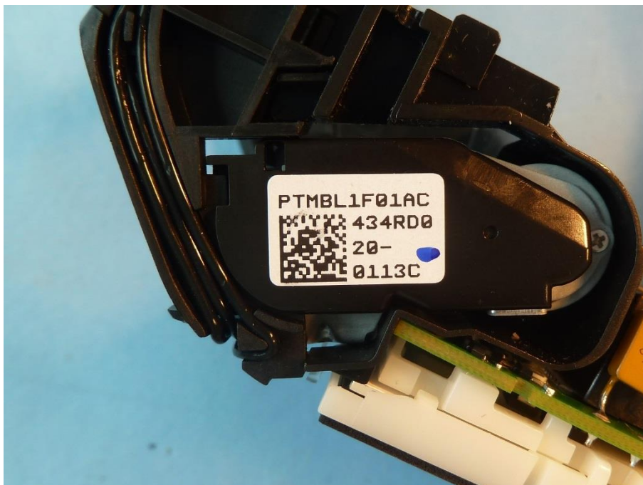
Photo 6: antenna (wire loop antenna)
