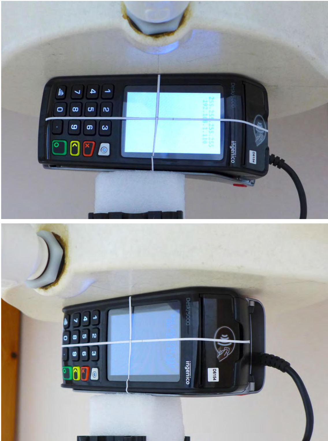
Pic. 4: Test position – left side, 0mm distance to phantom.
