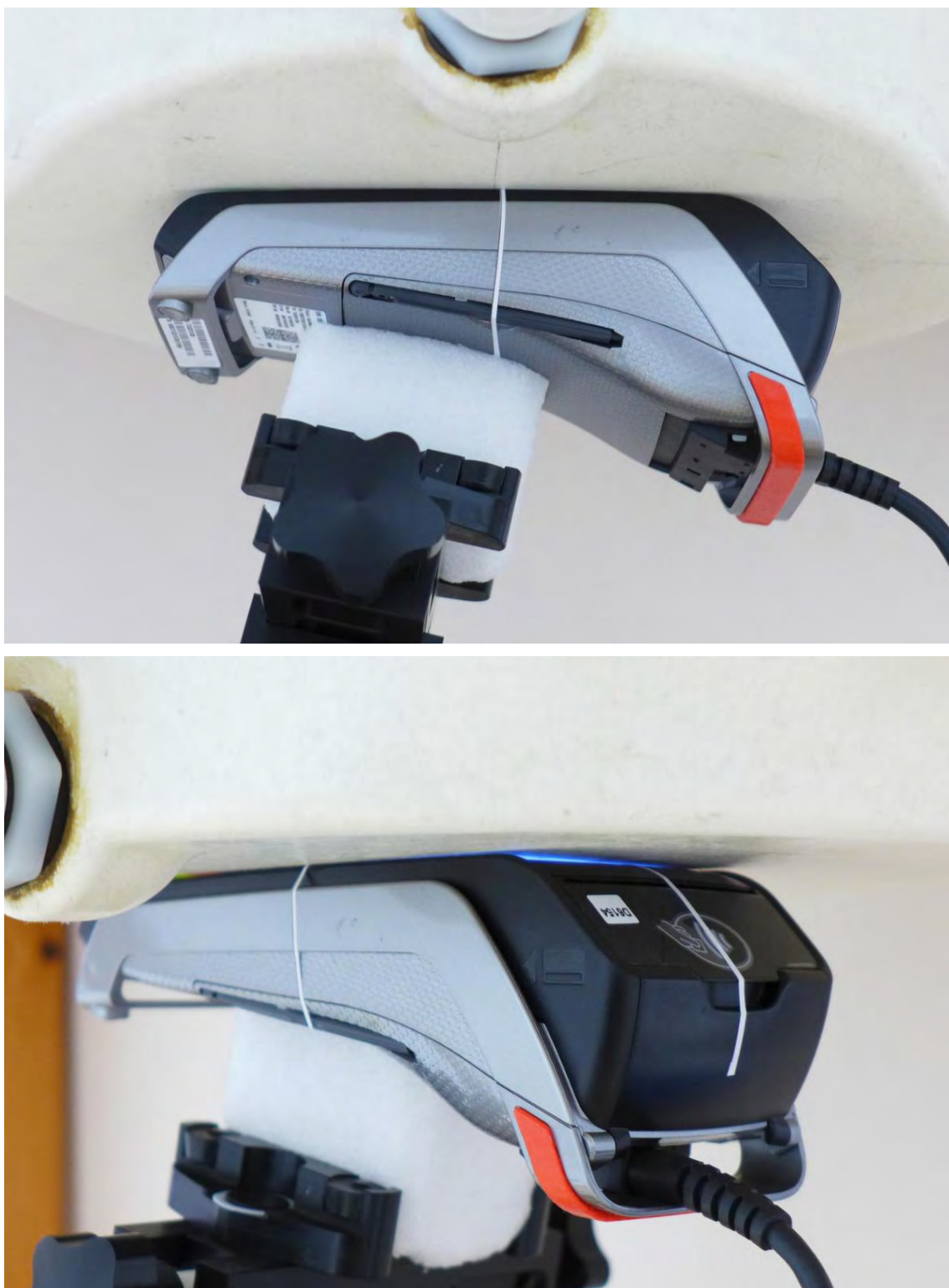
Pic. 3: Test position – front side, 0mm distance to phantom.
