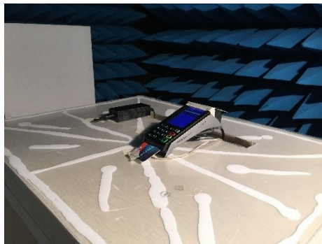
Test setup in anechoic chamber (Above 1GHz)
