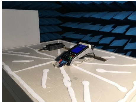
Test setup in anechoic chamber (Above 1GHz)
