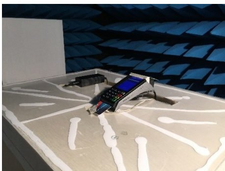
Test setup in anechoic chamber (Above 1GHz)
