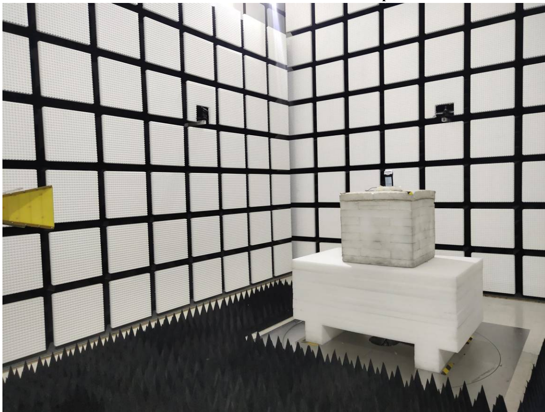
Radiated Emission Above 1GHz View Adapter 4#
