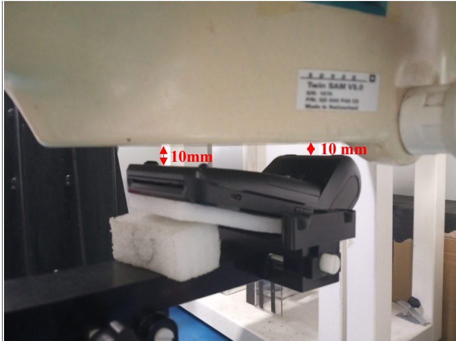
WWAN Body Back Setup Photo(10mm)
