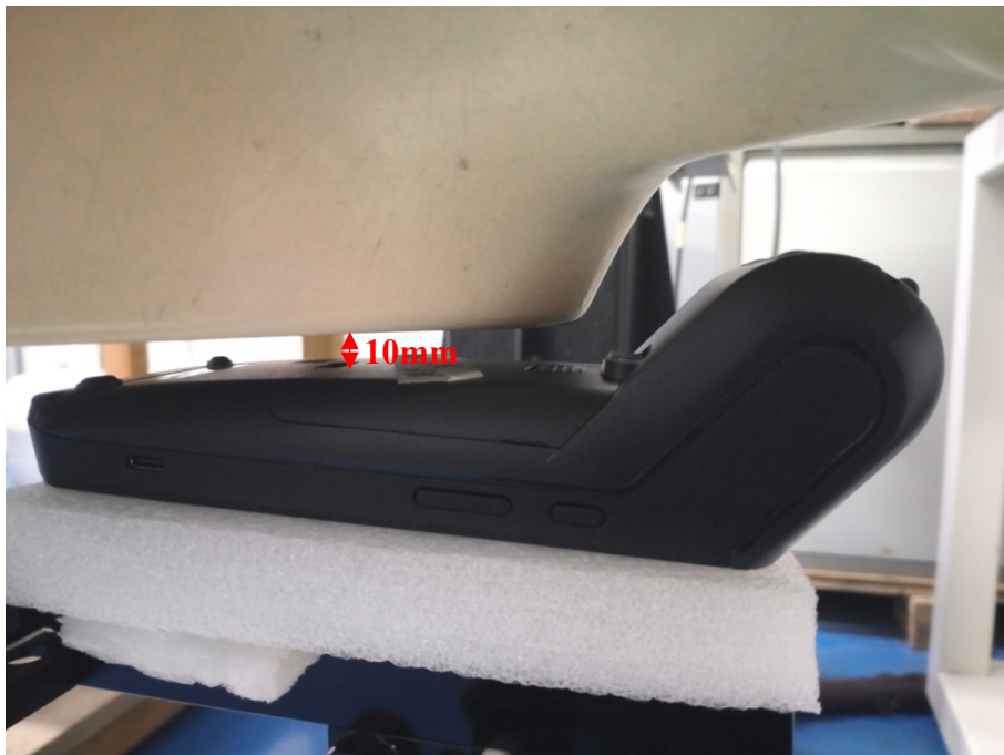
WLAN Body Back Setup Photo(10mm)
