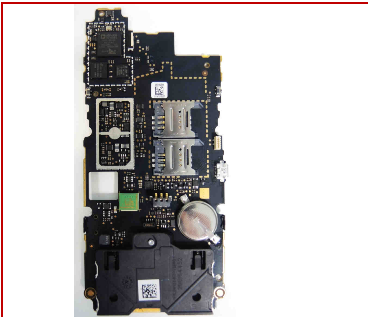
Figure #10 : Bottom side of the Main board
