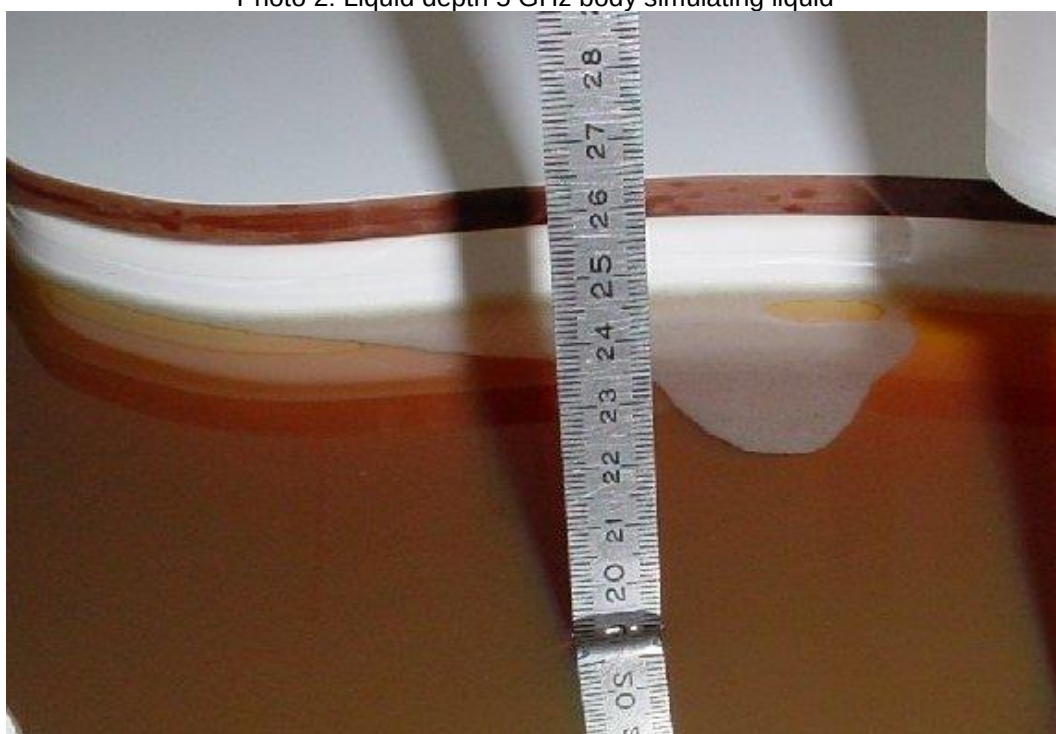
Photo 2: Liquid depth 5 GHz body simulating liquid
