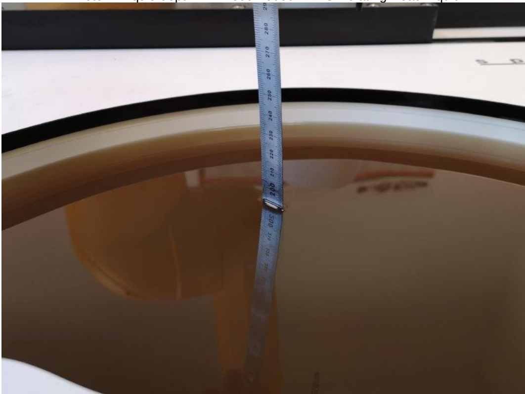
Photo 2: Liquid depth HBBL600-10000MHz Simulating Head Liquid
