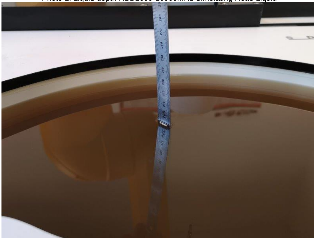
Photo 2: Liquid depth HBBL4-250V3 – 13MHz Simulating Head Liquid
