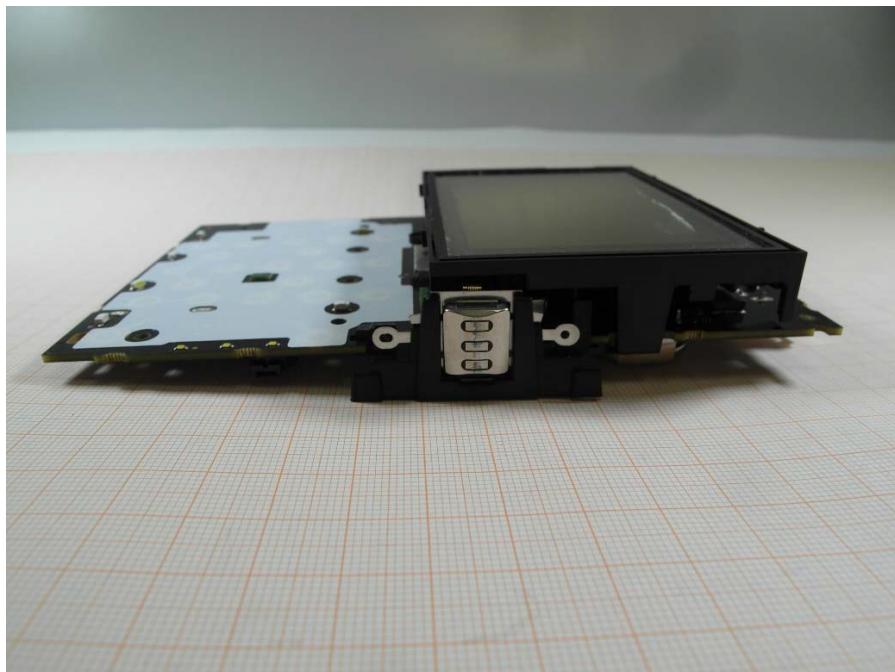
Photo 3: view on PCB with display and card reader
