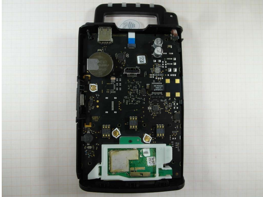
Photo 3: PCB with RF module in the bottom
