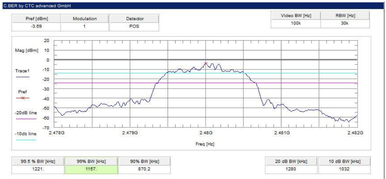
Plot 6: highest channel – 2480 MHz, Pi / DQPSK modulation
