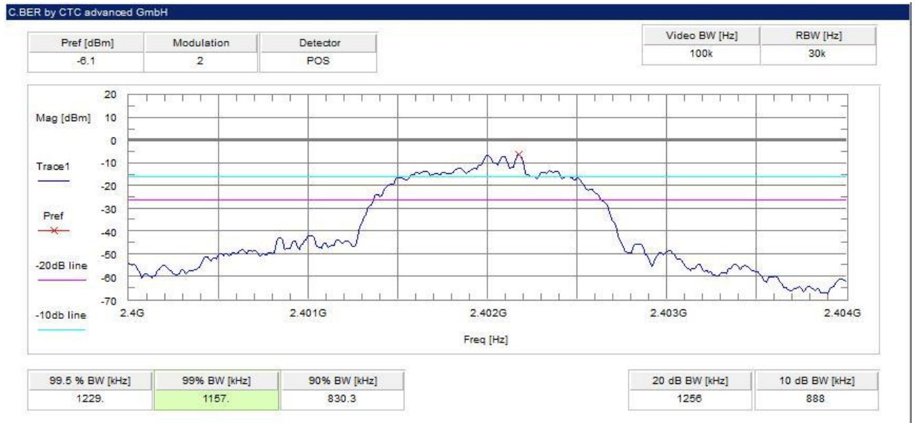
Plot 7: lowest channel – 2402 MHz, 8 DPSK modulation
