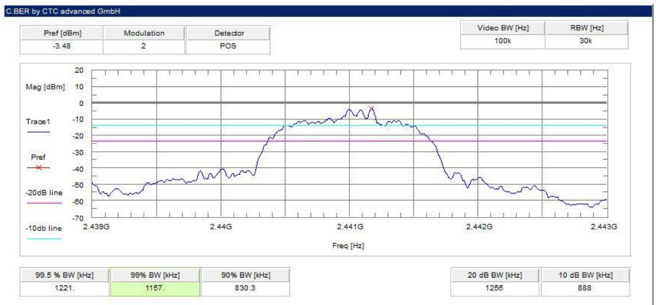
Plot 8: middle channel – 2441 MHz, 8 DPSK modulation
