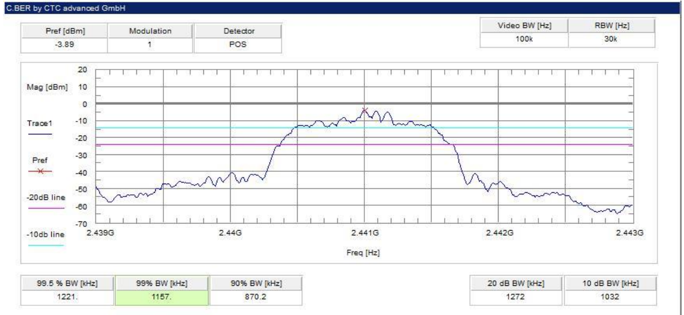
Plot 5: middle channel – 2441 MHz, Pi / DQPSK modulation
